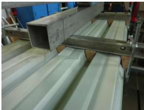
Figure 1.3.1 – Single span test on profile without a hole
