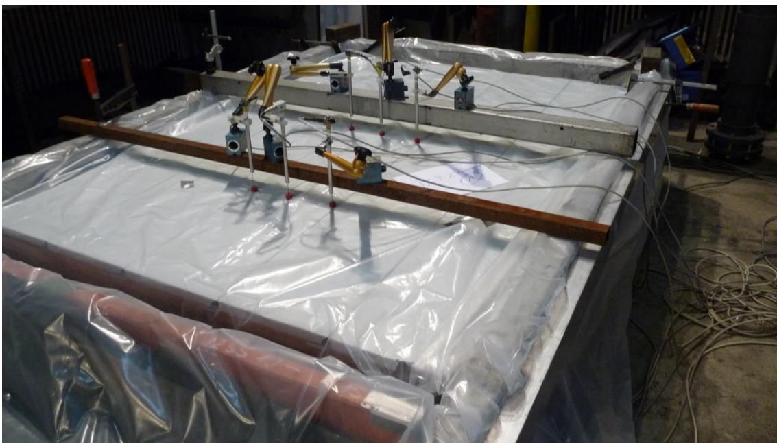
Figure 1.5 Test sample positioned on the vacuum chamber (pressure loads set-up)
