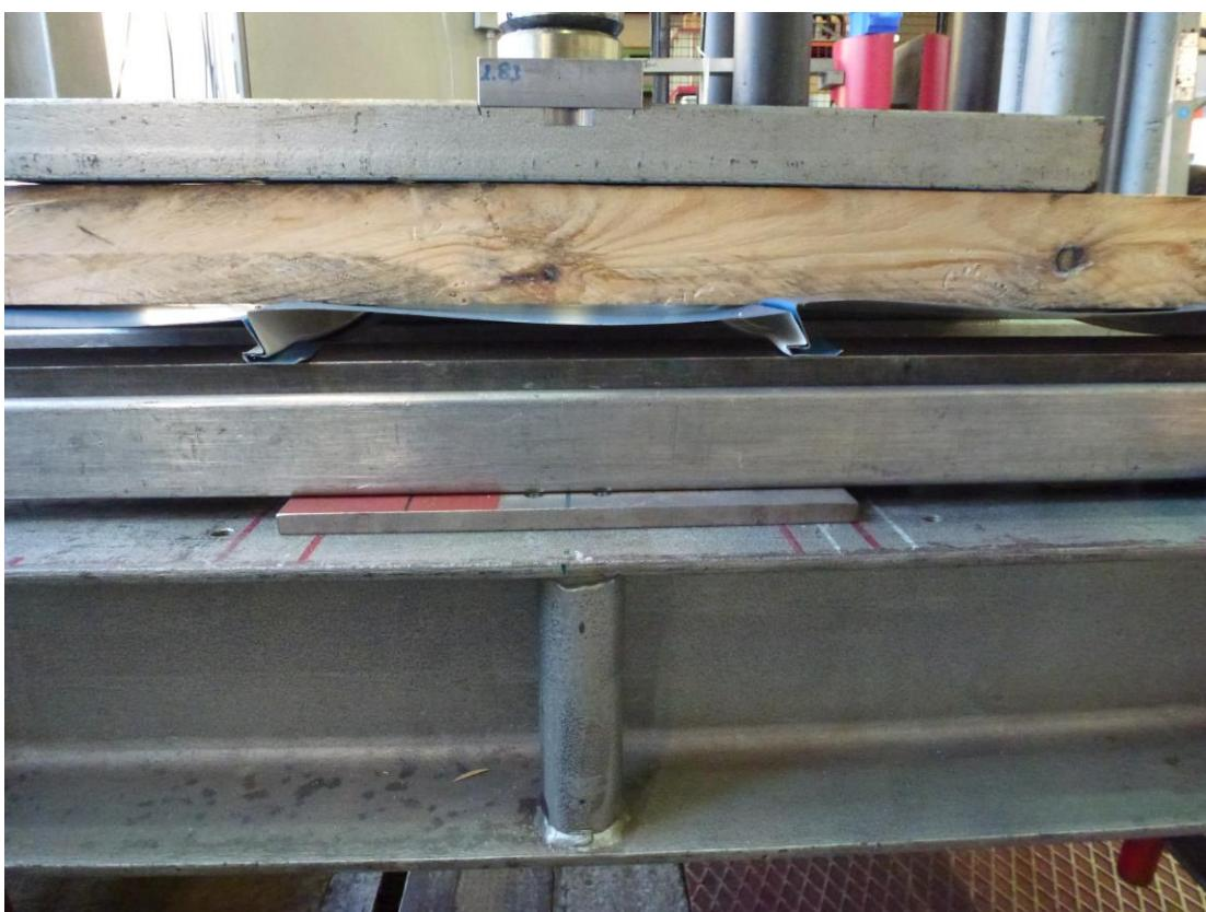
Fig. F.4: Web-crippling (Cladeo)
