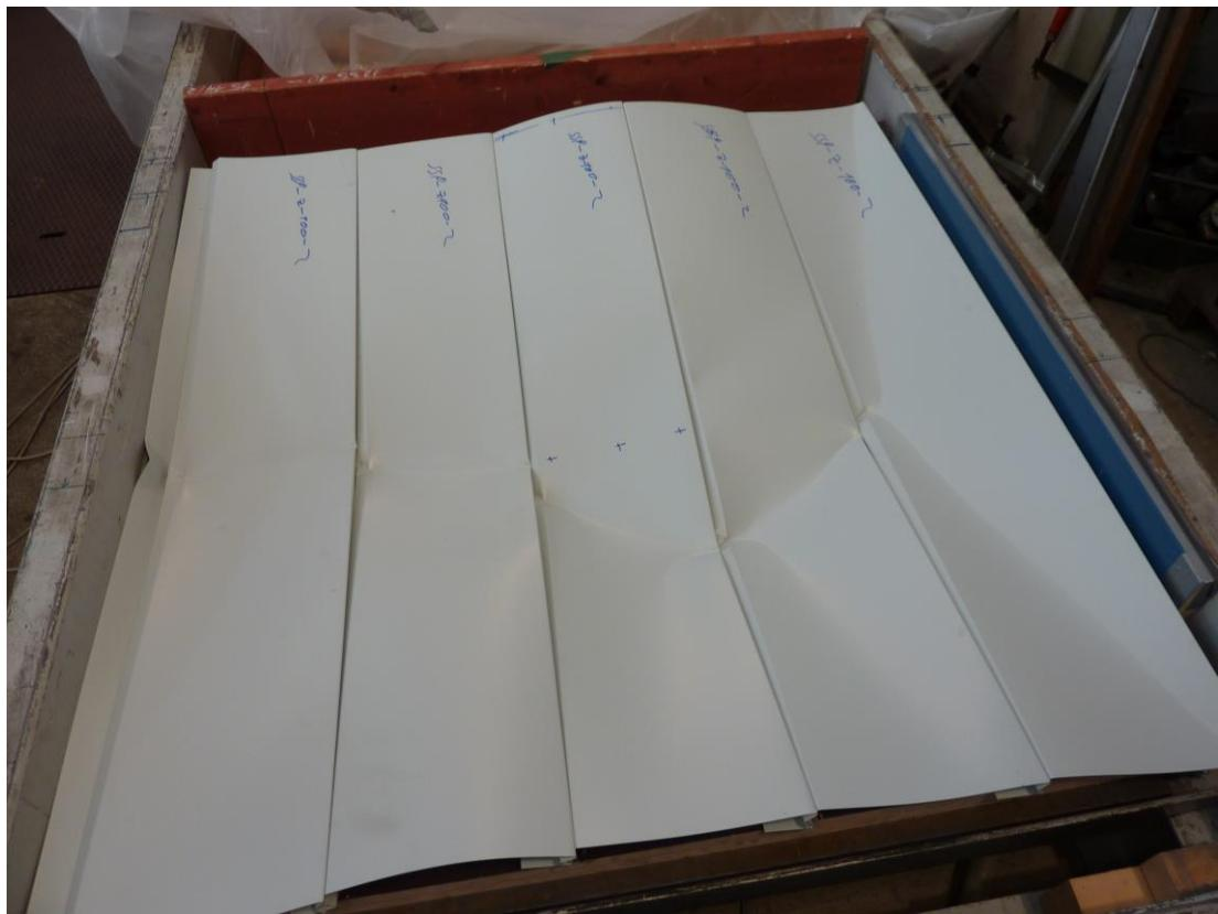
Fig. B.7: Failure mode (local buckling of the compressed flange, Zephyr  $t_N = 1.00$  mm)
