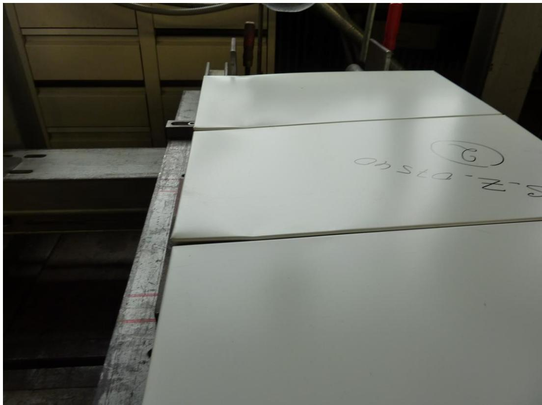
Fig. F.7: Local buckling under the load applying traverse (Zephir)
