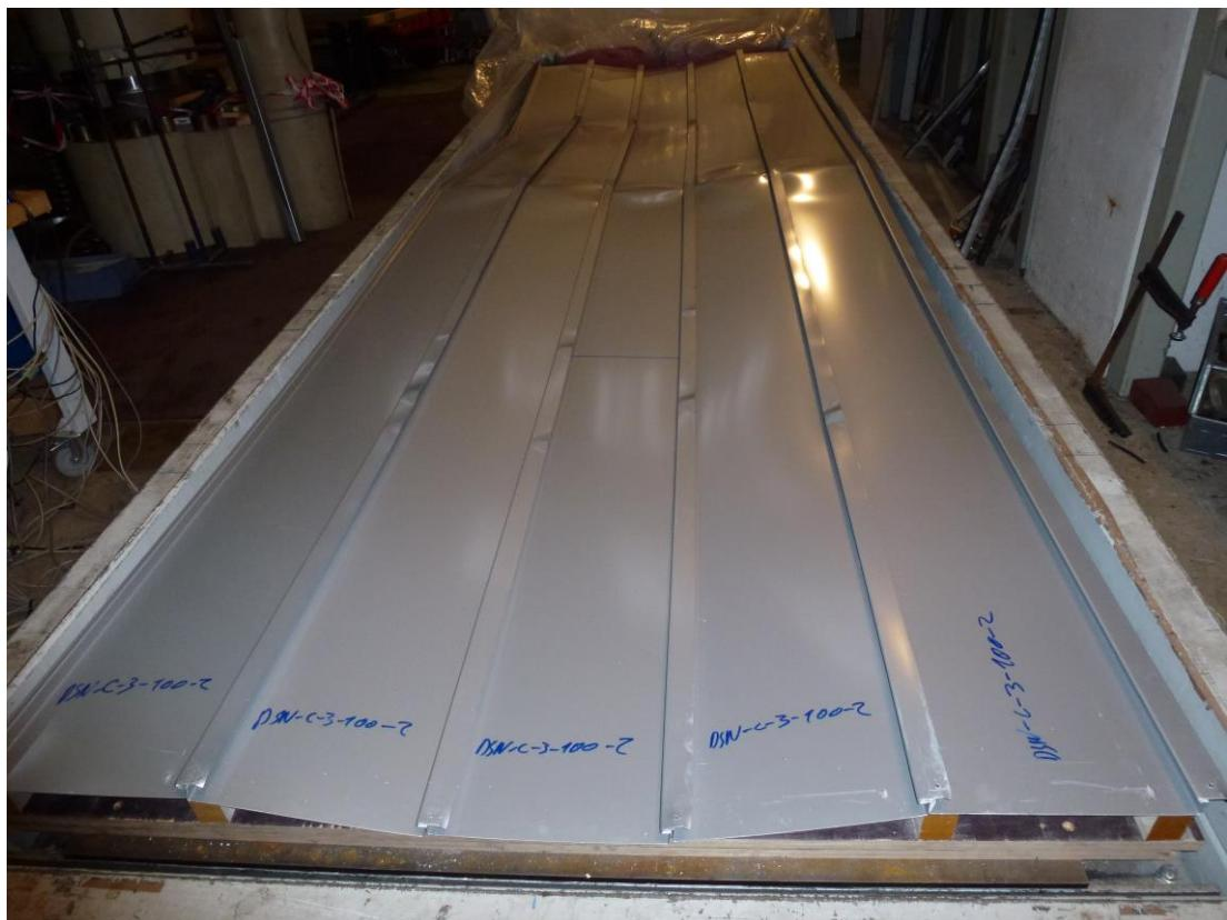
Fig. E.5: Failure by local buckling of the compressed flanges
