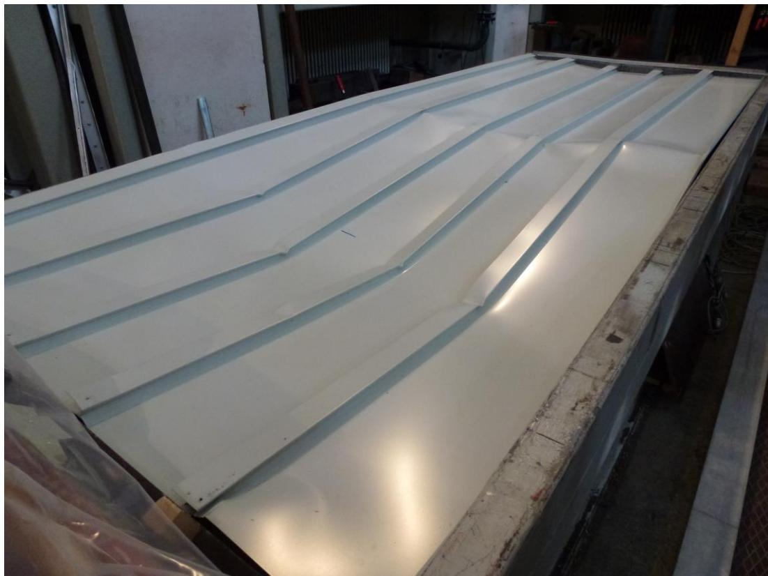
Fig. E.6: Failure by local buckling of the compressed flanges (DSN-Z-2-075-2)
