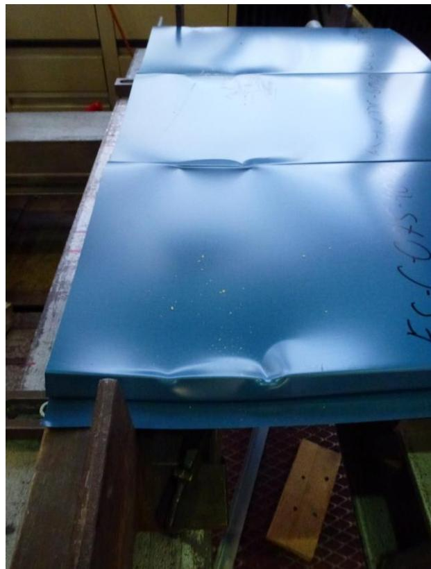
Fig. F.5: Local buckling under the load applying traverse (Cladeo)
