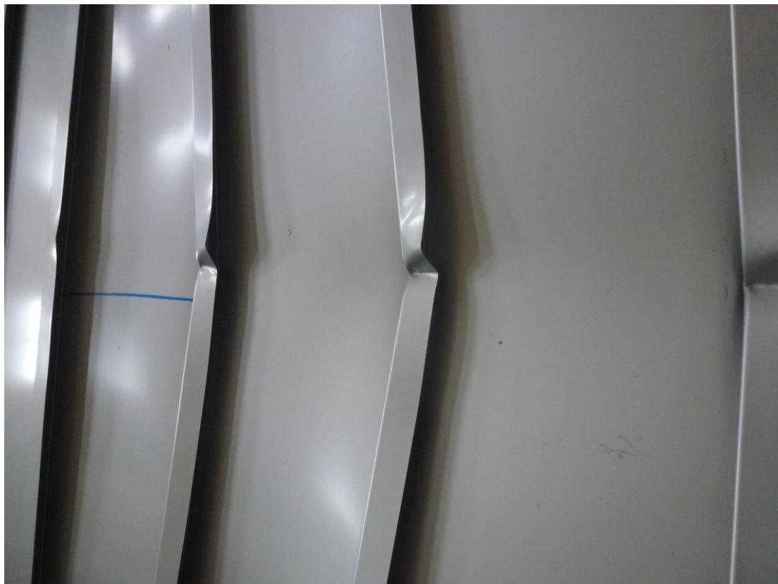
Fig. C.6: Failure mode (local buckling of the compressed flanges) of SSN-C-100-3
