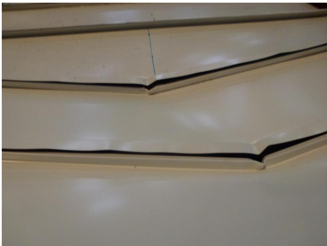
Fig. C.3: Failure mode (local buckling of the compressed flanges) of SSN-Z-075-3
