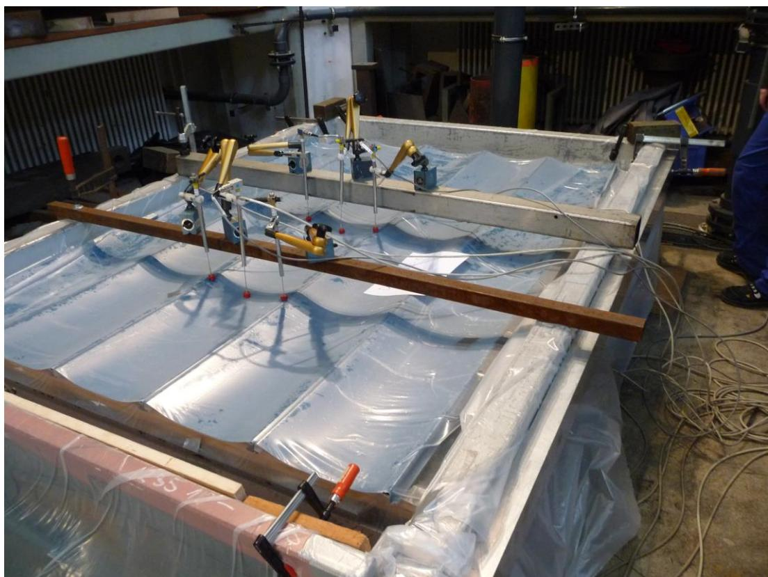
Fig. D.4: Deformation when maximum load of the vacuum chamber was reached (DSP-C-1-075-1)
