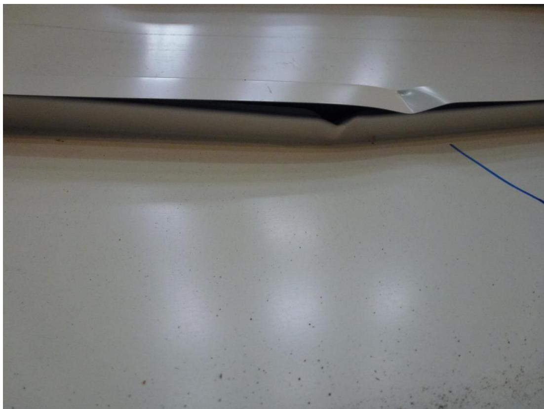
Fig. E.7: Failure by local buckling of the compressed flanges (DSN-C-1-075-2)
