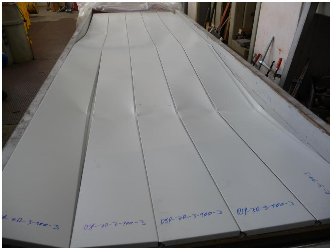
Fig. D.10: Failure by local buckling of the compressed flanges (DSP-ZR-3-100-3)
