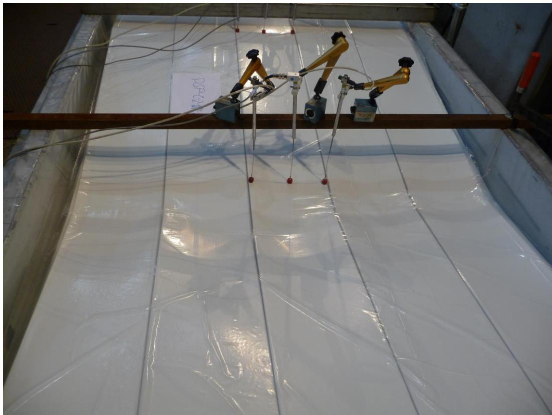
Fig. D.6: Failure by local buckling of the compressed flanges (DSP-C-2-100-1)
