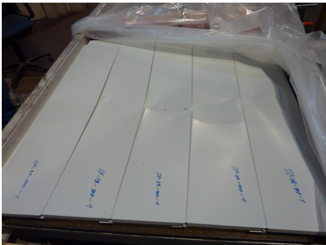
Fig. B.8: Failure mode (local buckling of the compressed flange, Zephyr  $t_N = 1.00$  mm)
