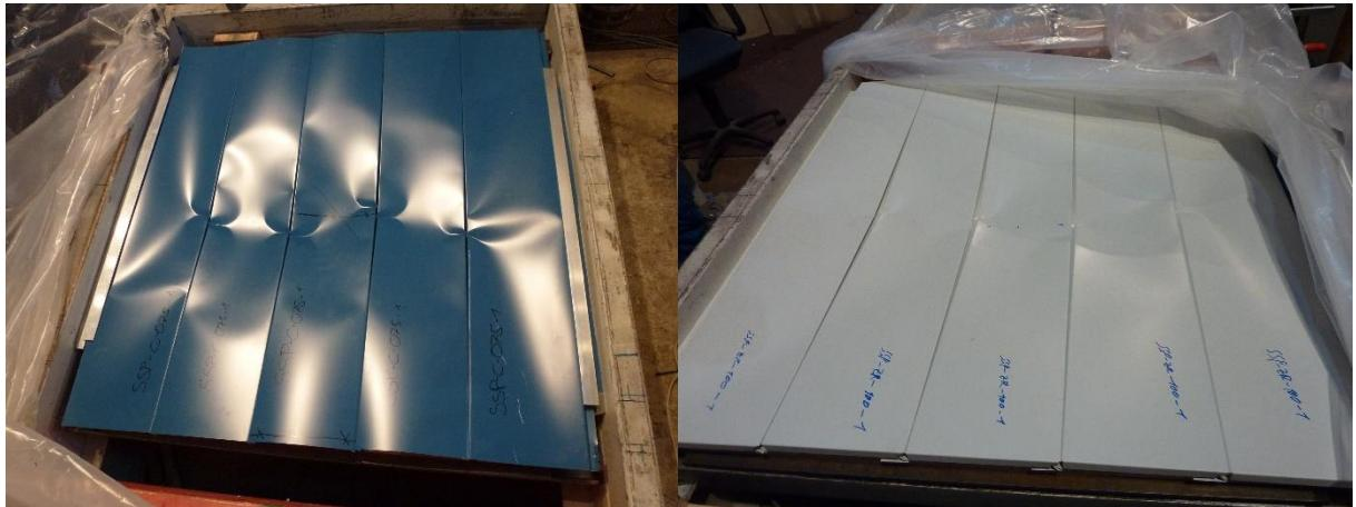
Figure 3 Failure by local buckling of the compressed flange (left: CLADEO 300  $t=0.75\text{mm}$  ; right ZEPHIR 300 with reinforcement  $t = 1 \text{ mm}$ )
