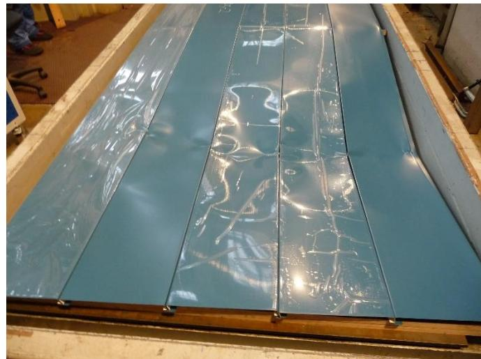
*Figure 10 Failure by local buckling (CLADEO 300 t = 0.75 mm)*
