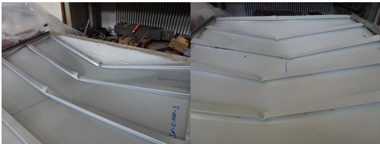
*Figure 6 Failure by local buckling of the compressed flange (left: CLADEO 300  $t=1.00\text{mm}$  ; right ZEPHIR 300 without reinforcement  $t = 0.75 \text{ mm}$ )*
