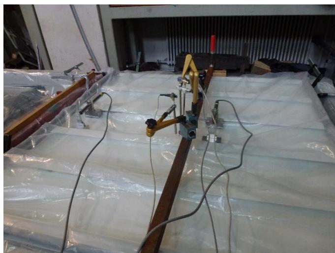
Figure 5 Test setup with horizontal displacement sensors
