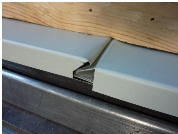
Figure 15 Failure by web crippling (end support tests)
