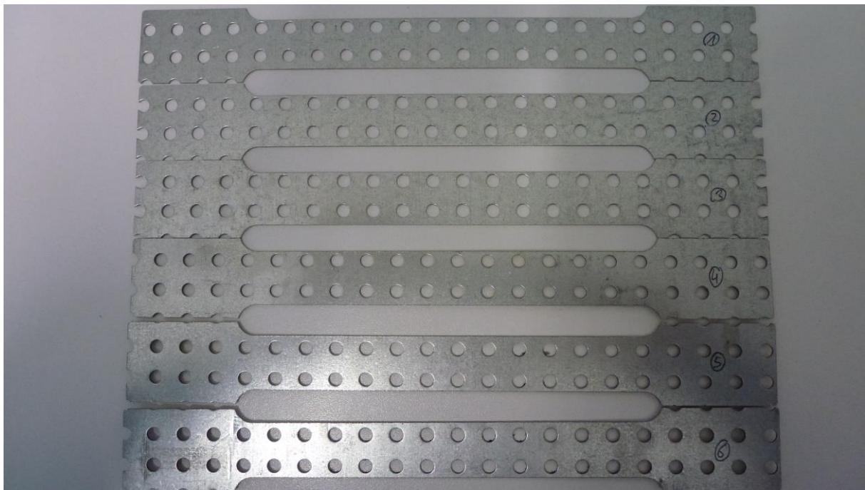
Fig. E.2: Tensile specimens with square perforation
