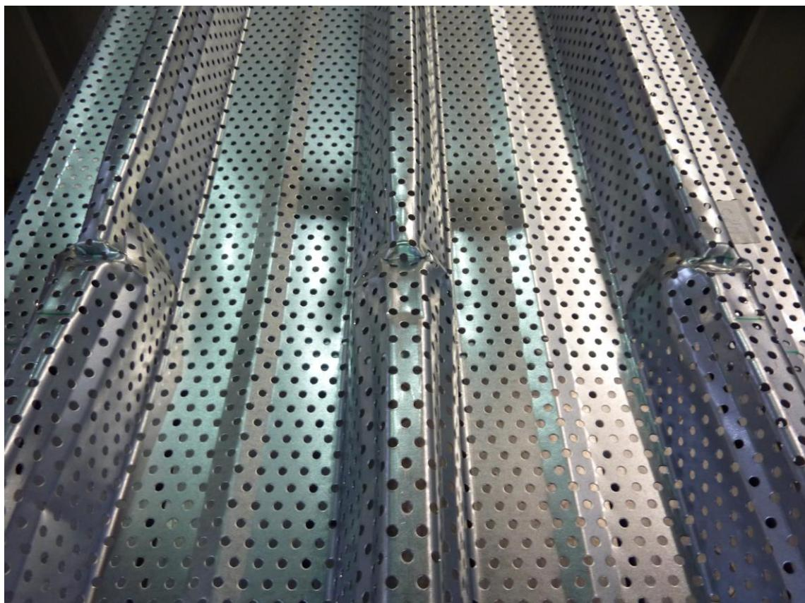
Figure C.12: Failure mode (exemplary for IS6-4t-triangle-075-42)
