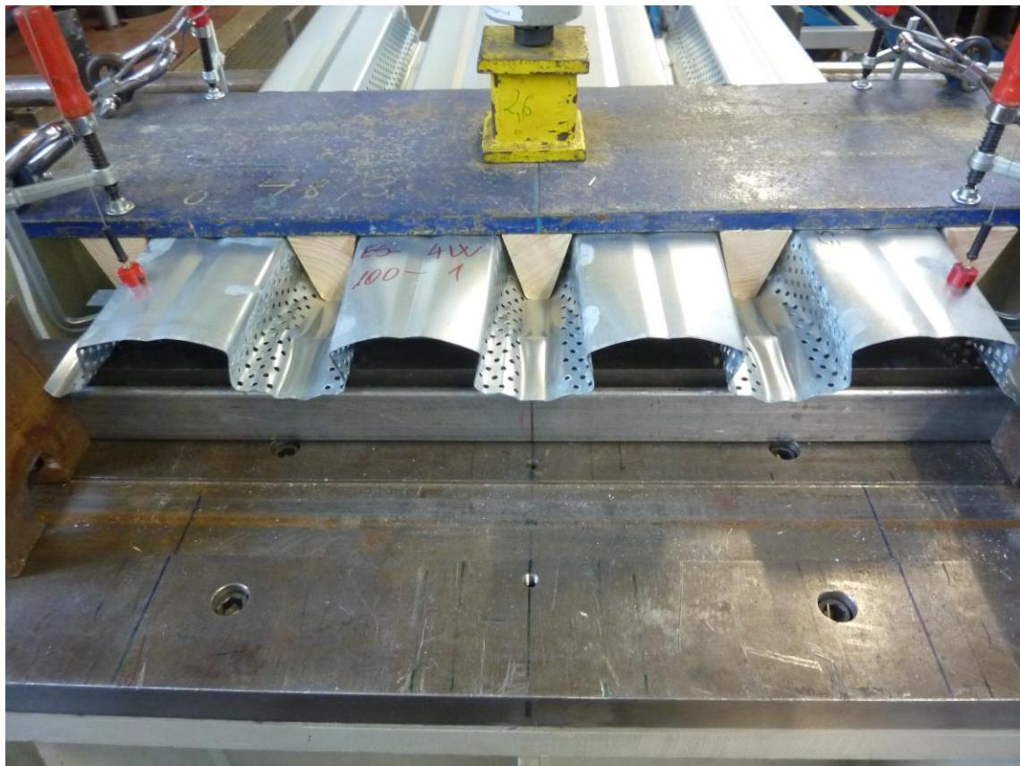
Figure D.4: Web-crippling (exemplary for ES-4w-triangle-100-1)
