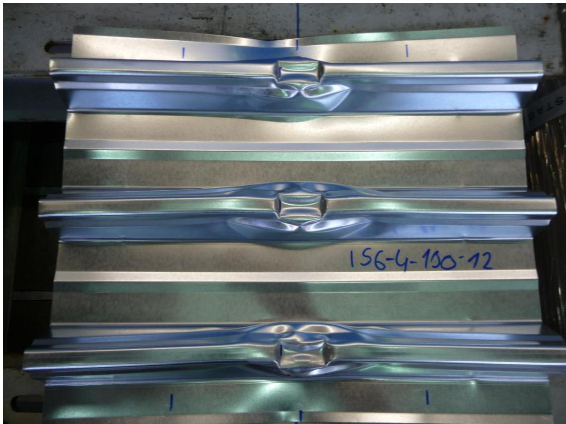
Figure C.13: Failure mode (exemplary for IS6-4-100-12)
