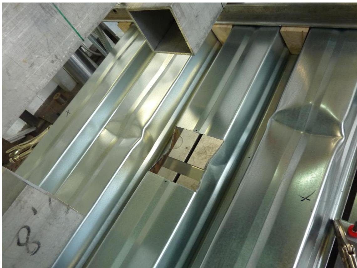
Figure B.7: Failure mode (exemplary for PF-4Hs1-075-1)
