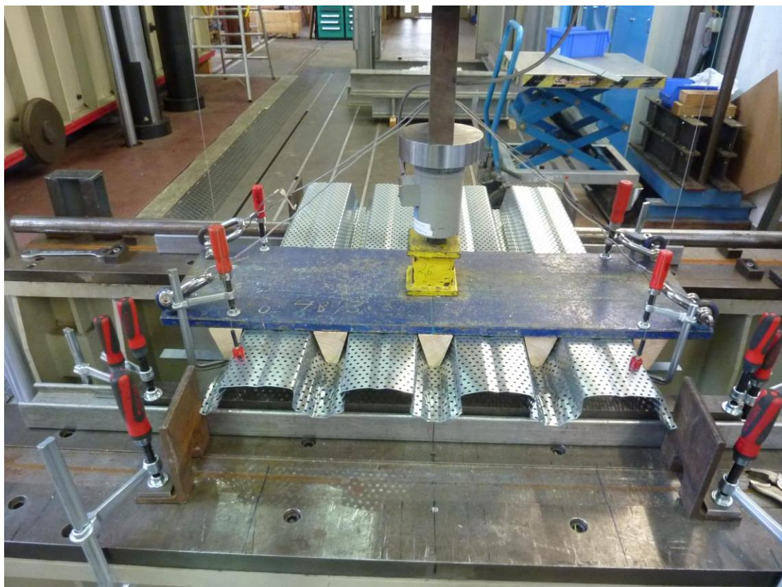
Figure D.5: Web-crippling (exemplary for ES-4t-triangle-075-2)
