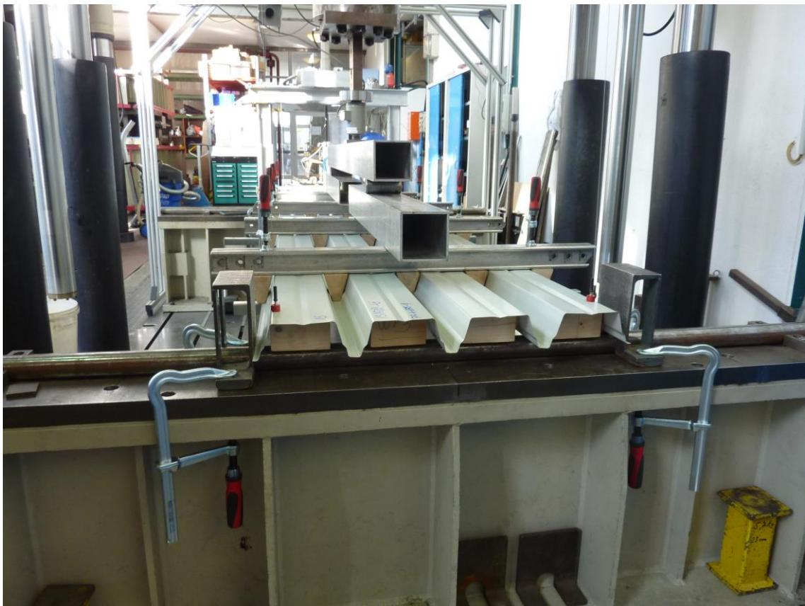
Figure B.2: Test setup (exemplary for PF-4-075-1)
