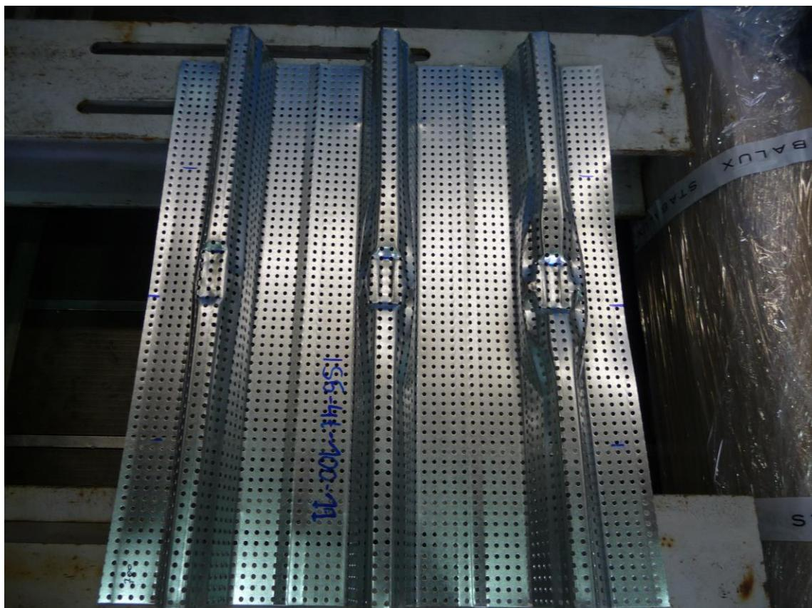
Figure C.16: Failure mode (exemplary for IS6-4-100-11)
