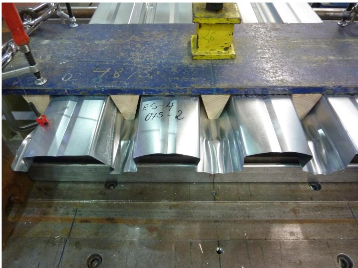
Figure D.7: Web-crippling (exemplary for ES-4-075-2)
