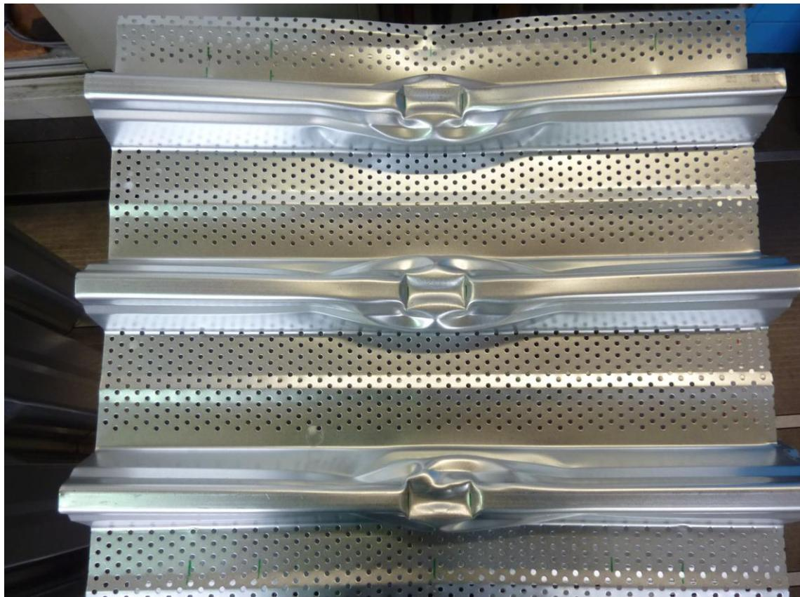
Figure C.6: Failure mode (exemplary for IS6-4f-100-11)
