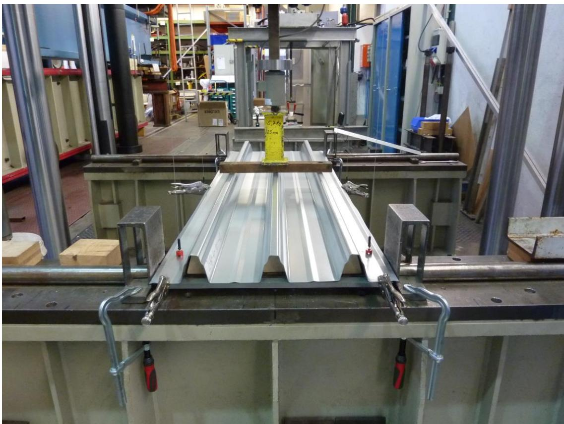
Figure C.4: Test setup (span s = 1700mm)
