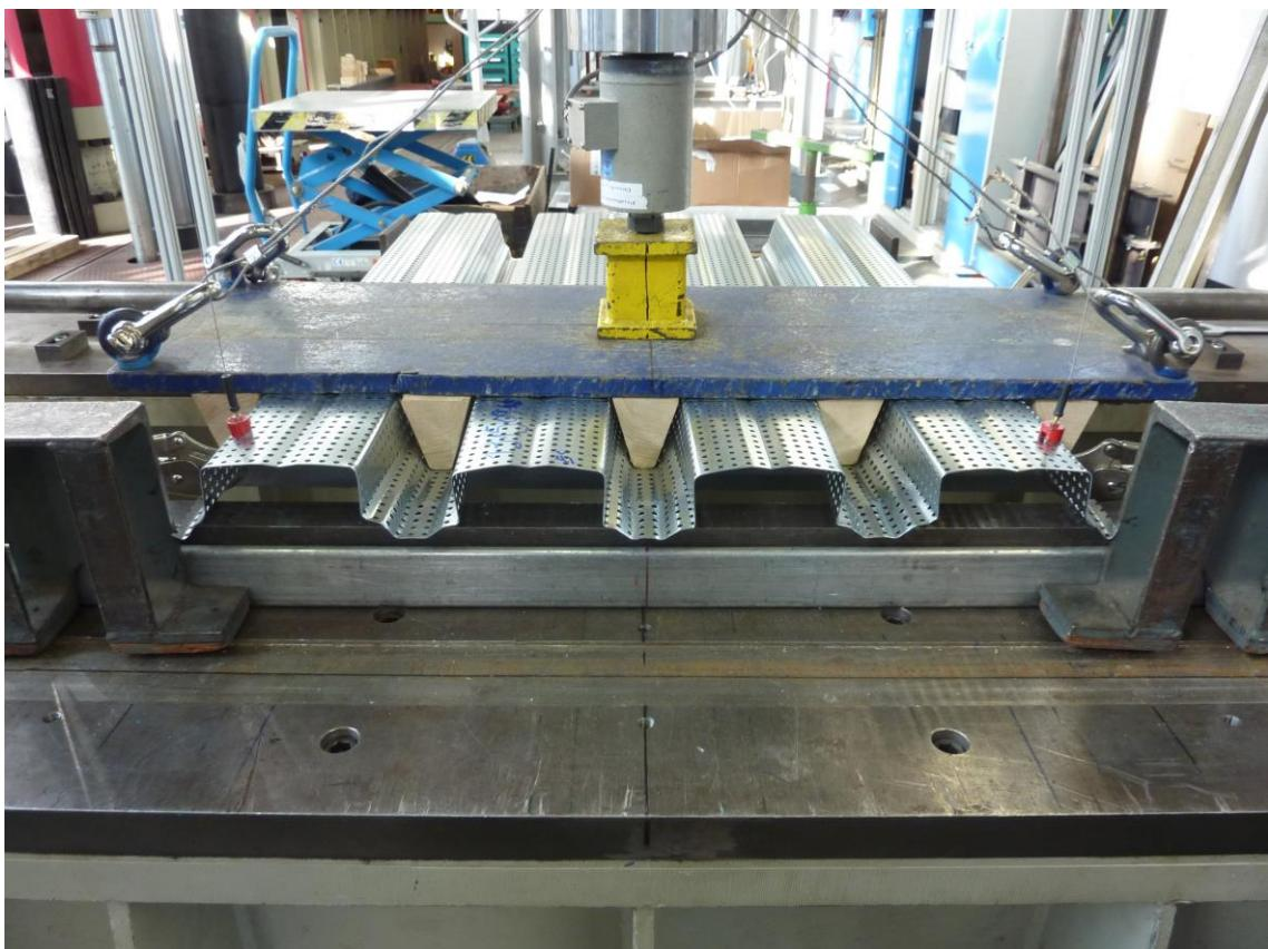
Figure D.11: Web-crippling (exemplary for ES-4t-075-1)
