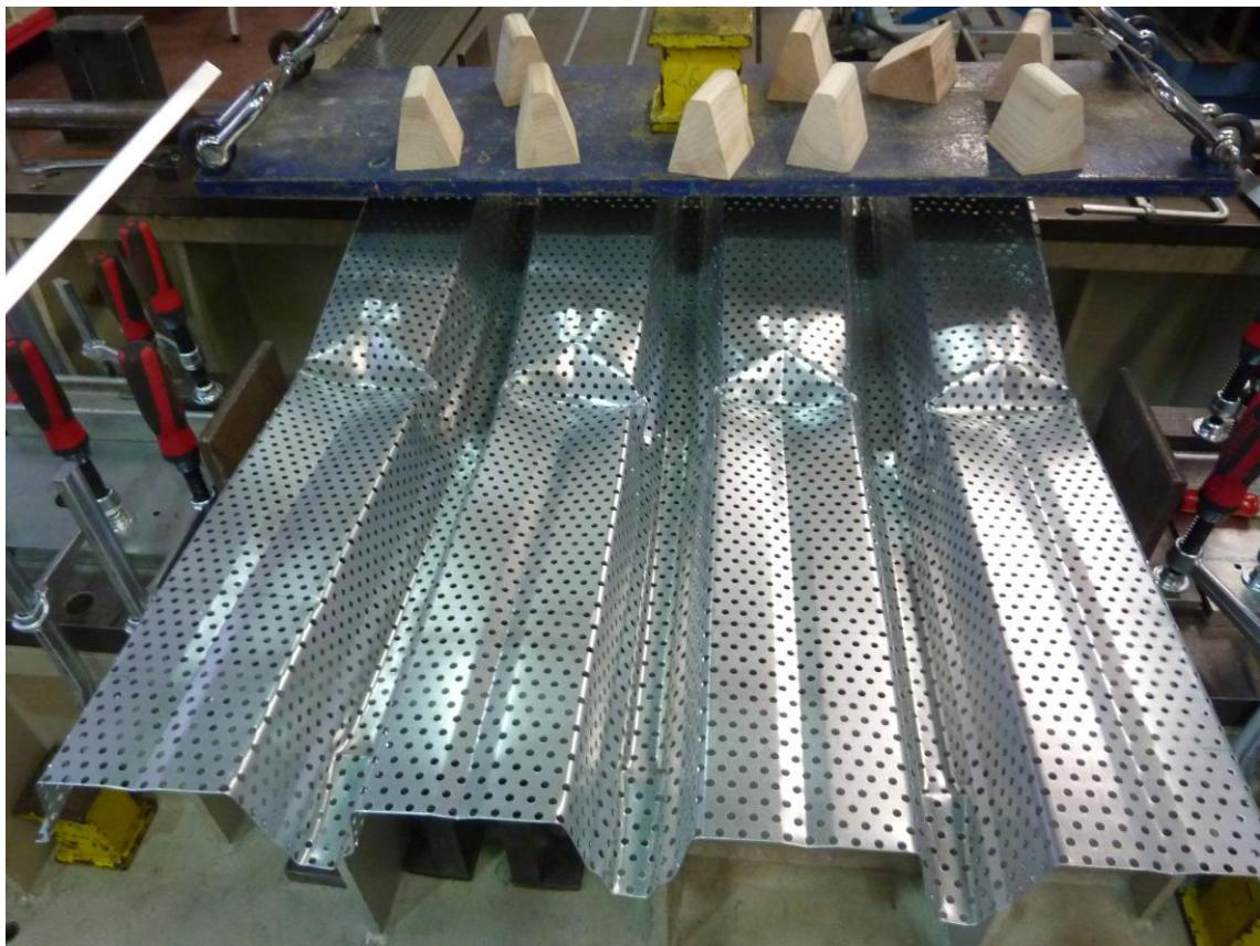
Figure D.6: bending failure under the load applying plate (exempl. for ES-4t-triangle-075-3)
