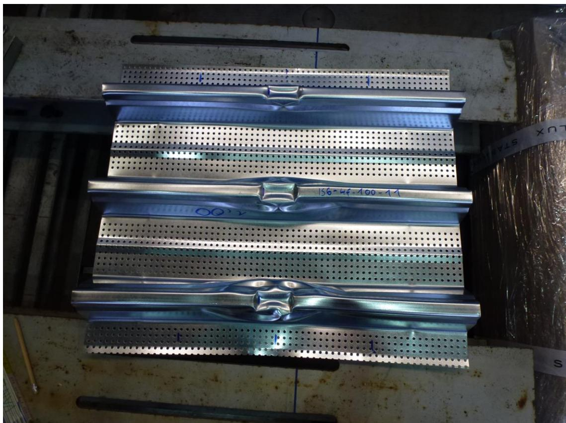
Figure C.14: Failure mode (exemplary for IS6-4f-100-11)
