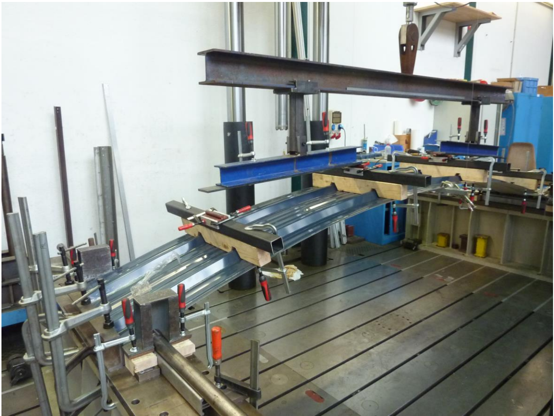
Fig. 10: Picture of the test setup single span test with horizontal support (profile 39/333)
