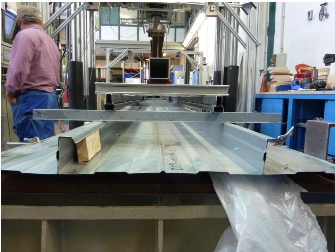
Figure D.15: Test setup for liner tray without outer cladding
