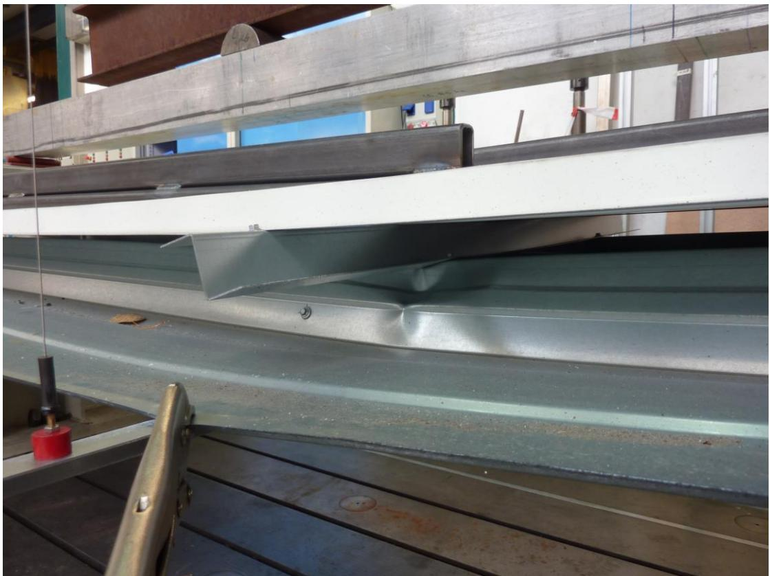
Figure D.6: Web crippling in the middle of the span under the Z-profile  $h = 50$  mm
