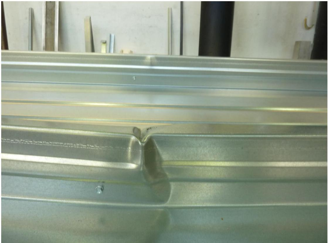
Figure B.6: Failure mode (buckling of the upper flange in the middle of the span, near the fixation of the flange)
