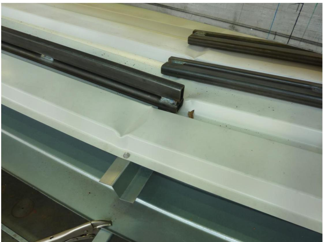
Figure D.9: Failure mode (buckling of the trapezoidal sheet in the middle of one span, Z-profile h = 50 mm), close up
