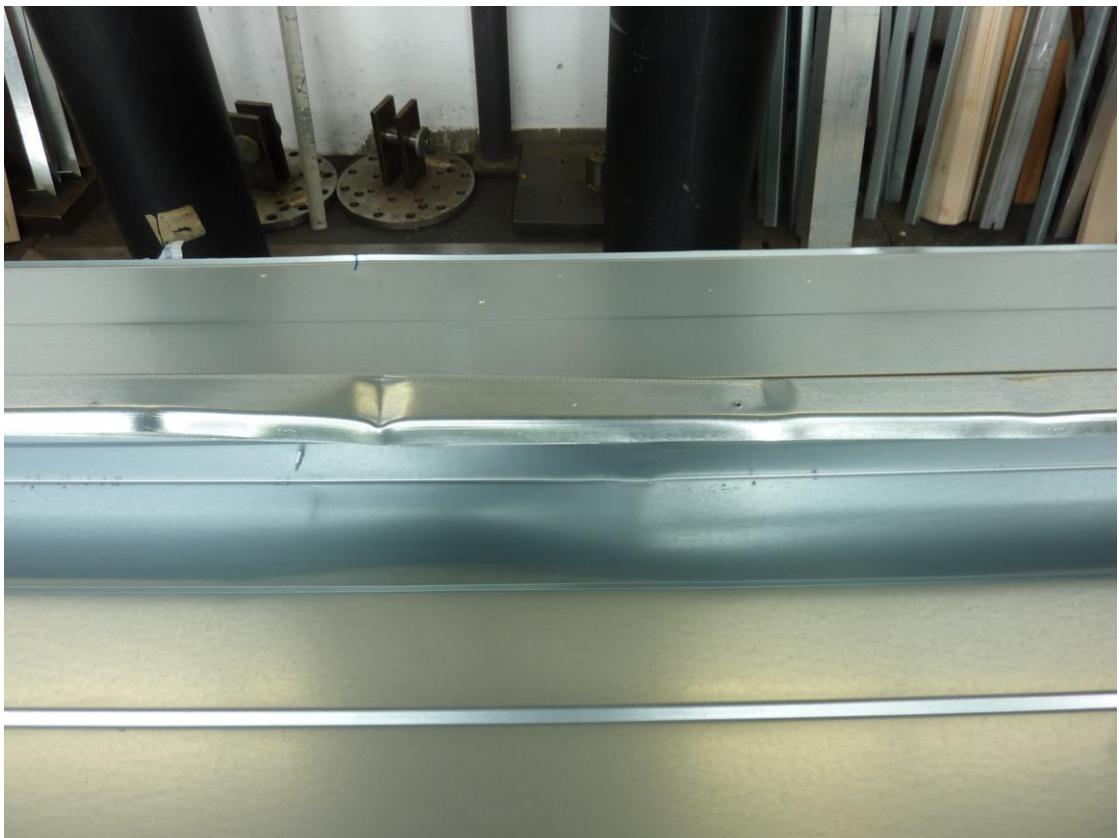
Figure B.5: Failure mode (buckling of the upper flange in the middle of the span, between two fixations of the flange)
