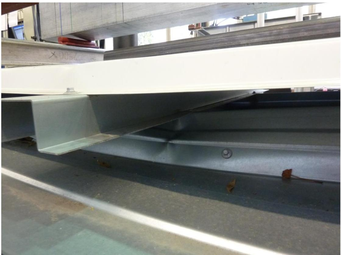
Figure D.11: Web crippling in the middle of the span under the omega-profile  $h = 50 \text{ mm}$
