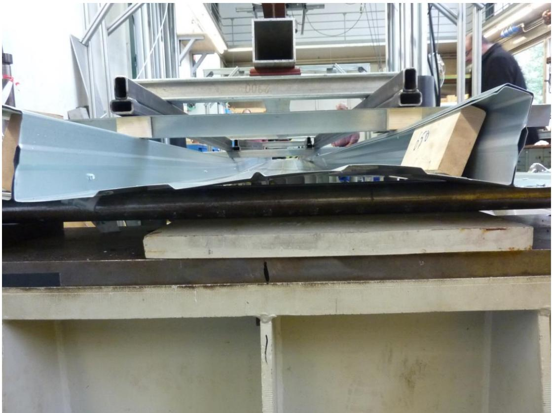
Figure D.16: Deformation of the lower flange of the liner tray at the maximum load (test without outer cladding)
