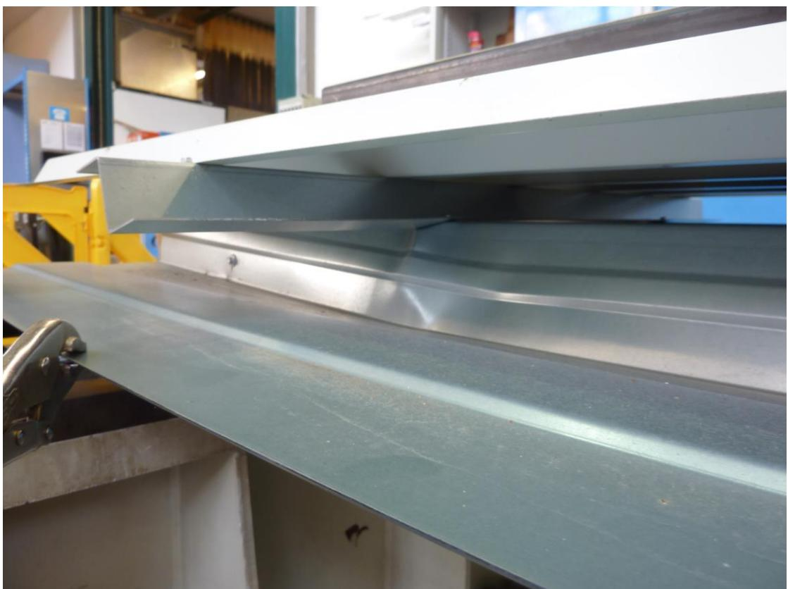
Figure D.5: Web crippling near the end support under the Z-profile  $h = 50$  mm
