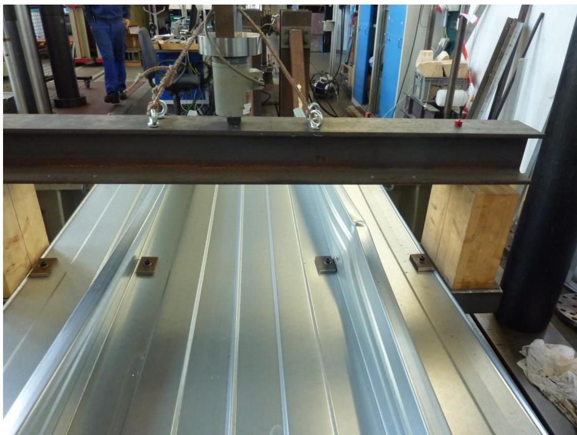
Figure C.6: Failure mode (liner tray without trapezoidal sheet)
