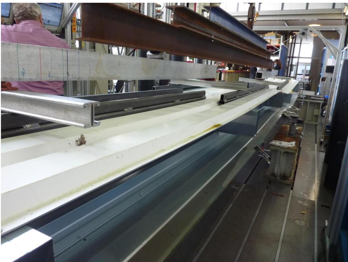
Figure D.13: Deformation of the test specimen near the maximum load (omega-profile  $h = 200$  mm)
