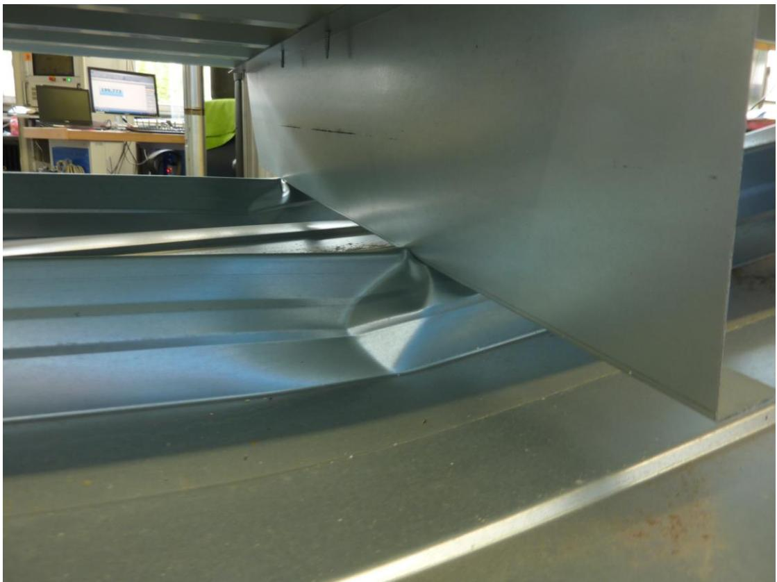
Figure D.4: Web crippling near the end support under the Z-profile  $h = 200$  mm
