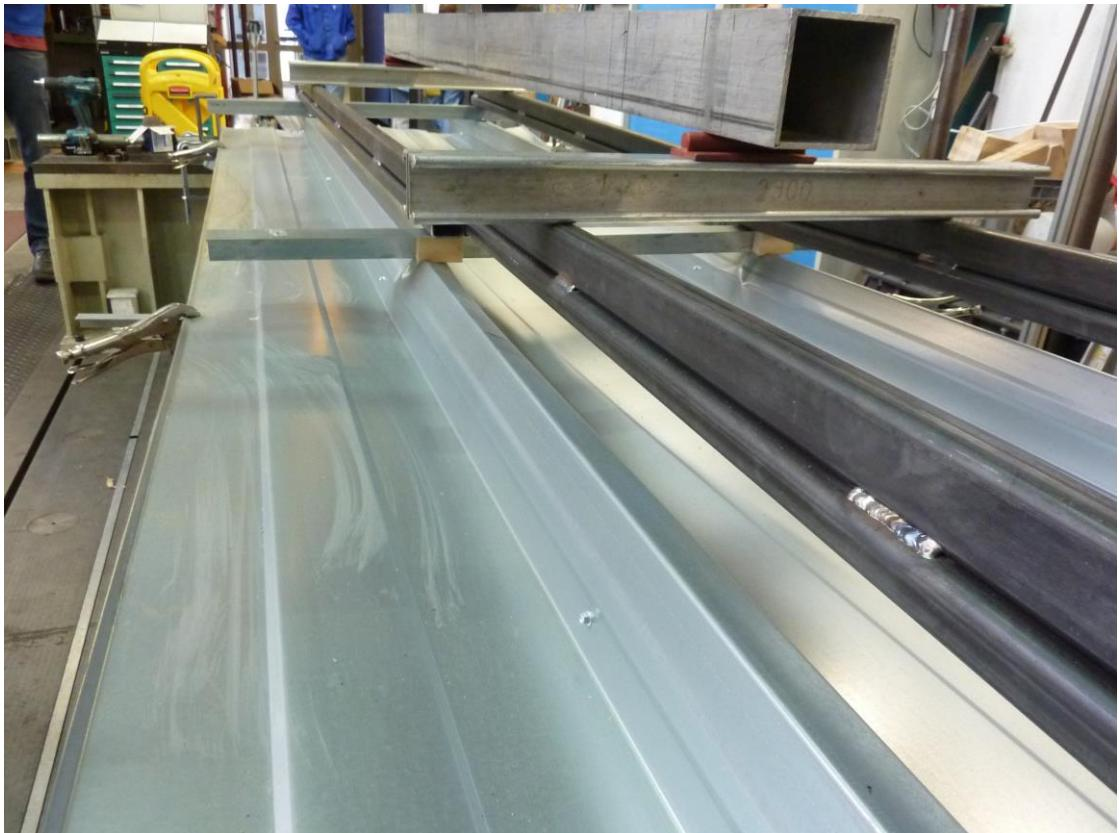
Figure D.17: Failure mode (torsional buckling of the upper flange in combination with web-crippling und the Z-profile h = 50 mm)
