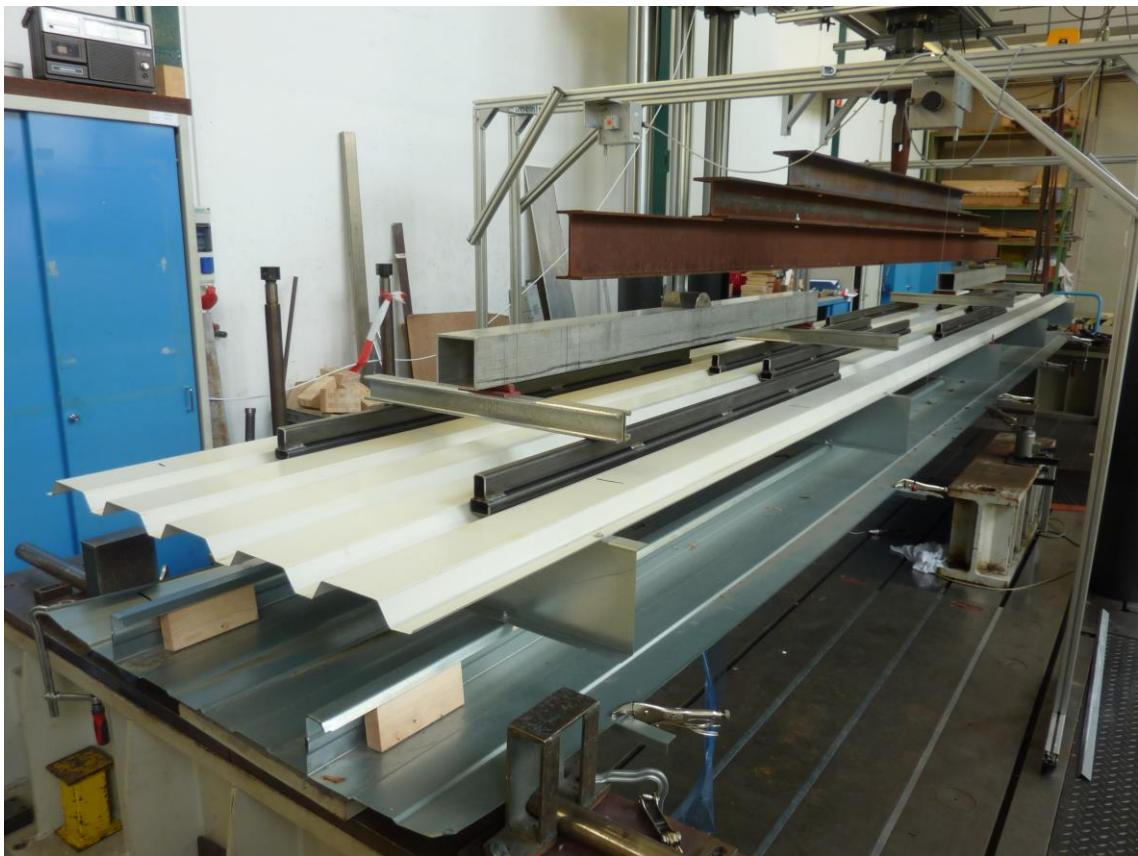
Figure D.2: Test setup (Z-profile  $h = 200$  mm)
