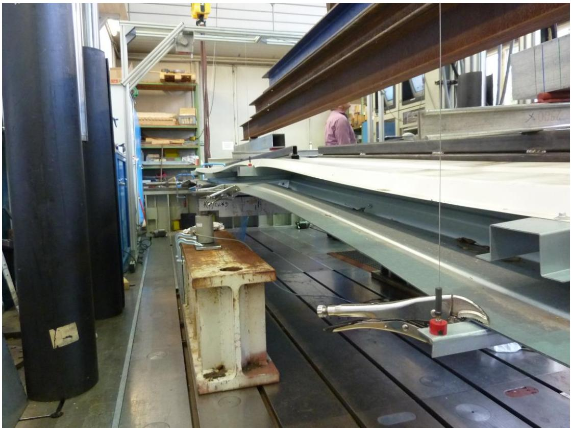
Figure D.10: Deformation of the test specimen near the maximum load (omega-profile
