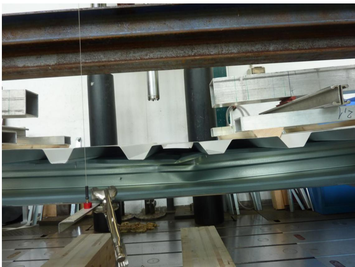
Figure B.4: Failure mode (buckling of the upper flange in the middle of the span)
