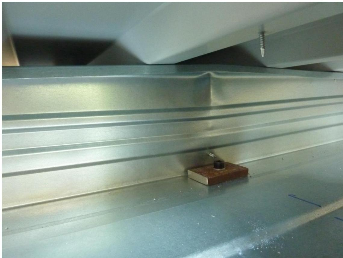
Figure C.5: Failure mode (buckling of the upper flange)
