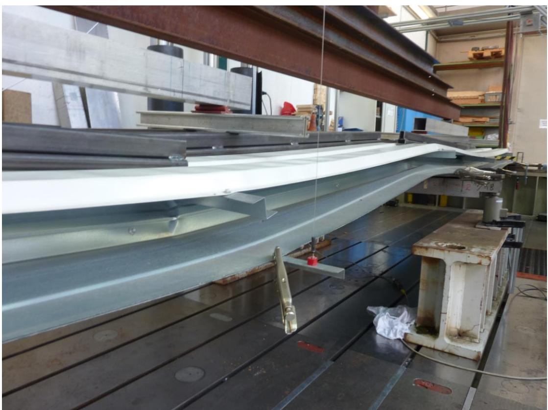
Figure D.7: Deformation of the test specimen at the maximum load (Z-profile  $h = 50$  mm)
