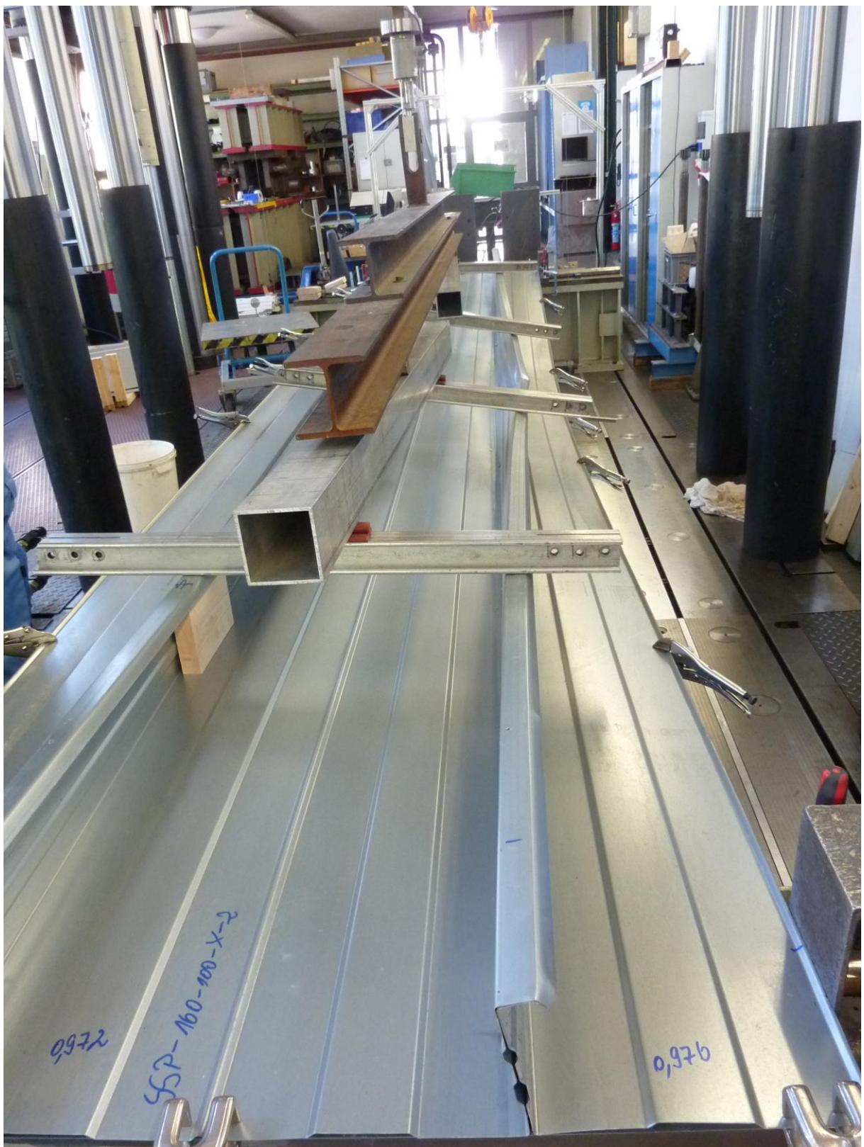
Figure B.11: Failure mode (liner tray without outer cladding, load distribution in the upper flange)
