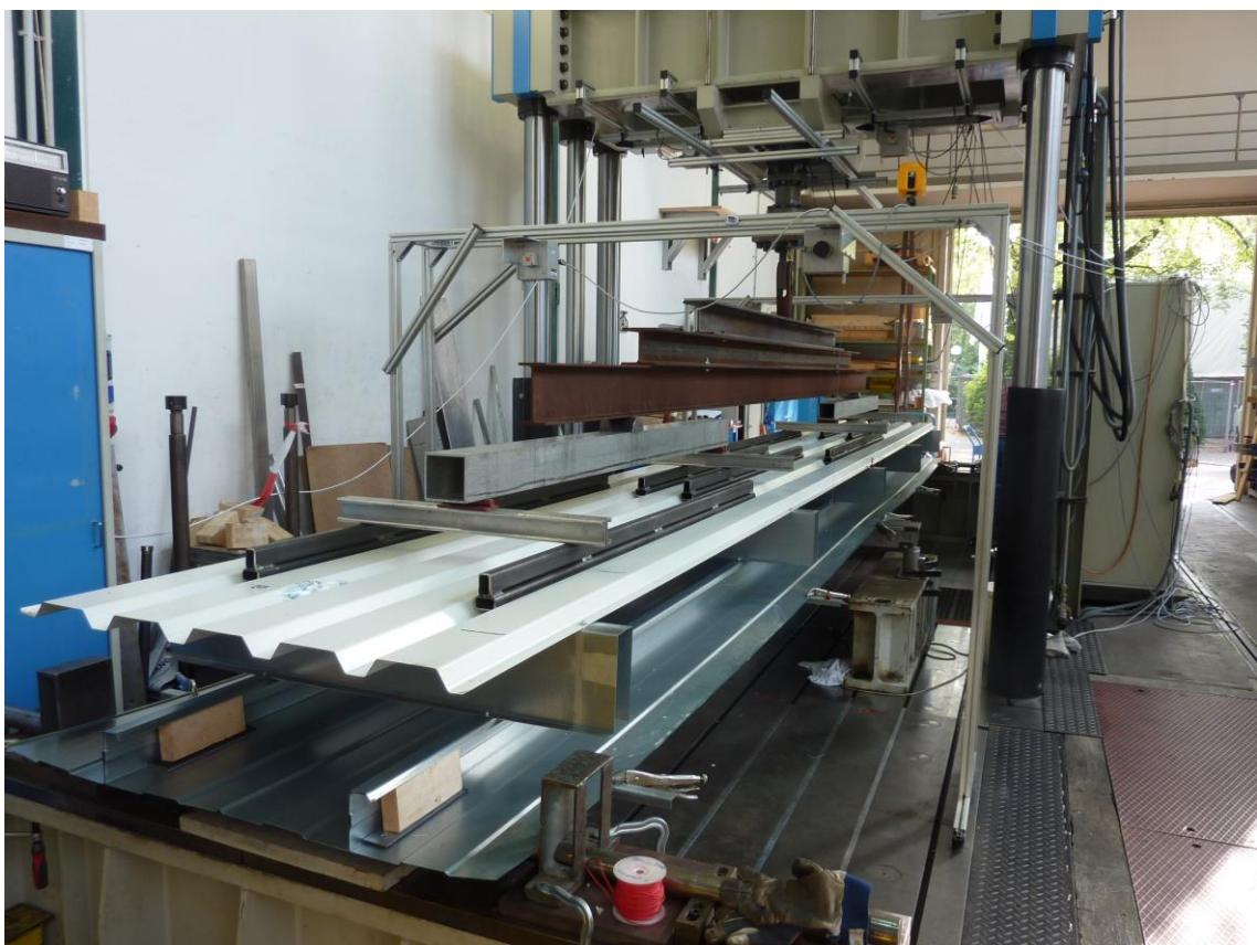
Figure D.3: Test setup (omega-profile  $h = 200$  mm)
