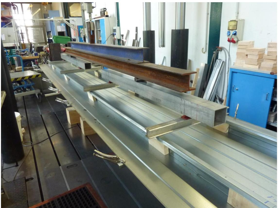
Figure B.8: Test setup (liner tray without outer cladding, load distribution in the upper flange)
