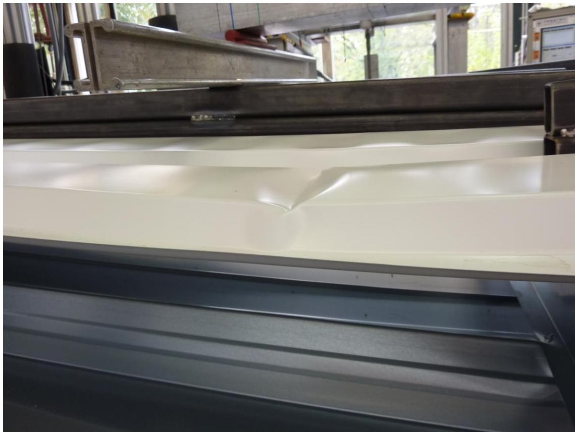
Figure D.14: Failure mode (buckling of the trapezoidal sheet in the middle of one span, omega-profile  $h = 200$  mm)
