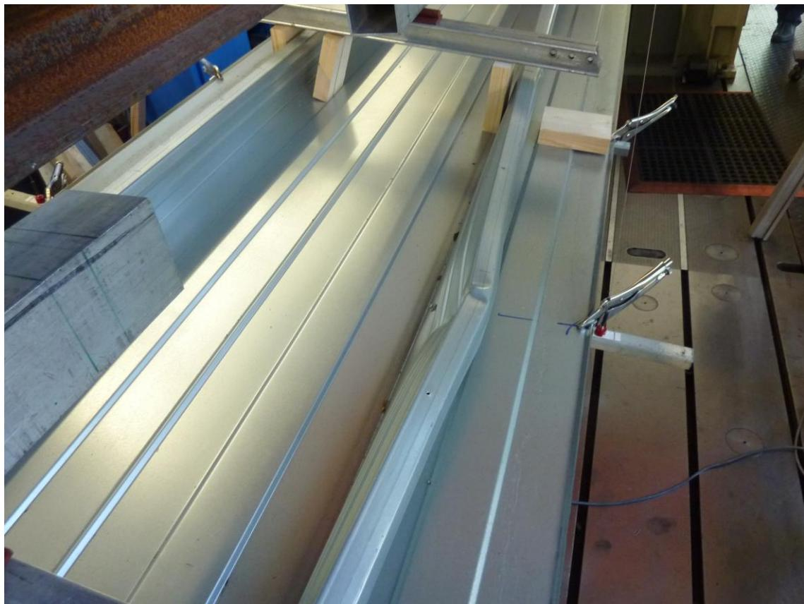
Figure B.9: Failure mode (liner tray without outer cladding, load distribution in the lower flange)
