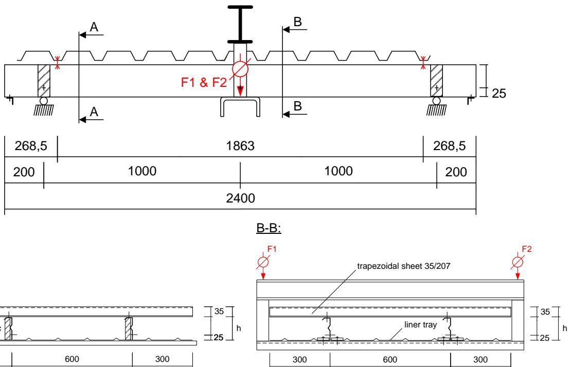
Figure C.3: Schematic test setup ( $s_1 = 1863$  mm)
