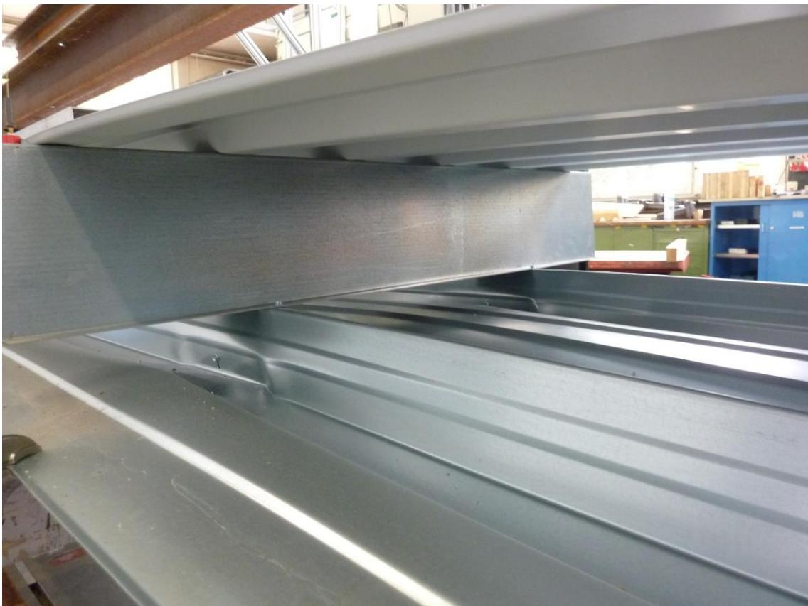
Figure D.12: Web crippling at the middle support under the omega-profile  $h = 200$  mm
