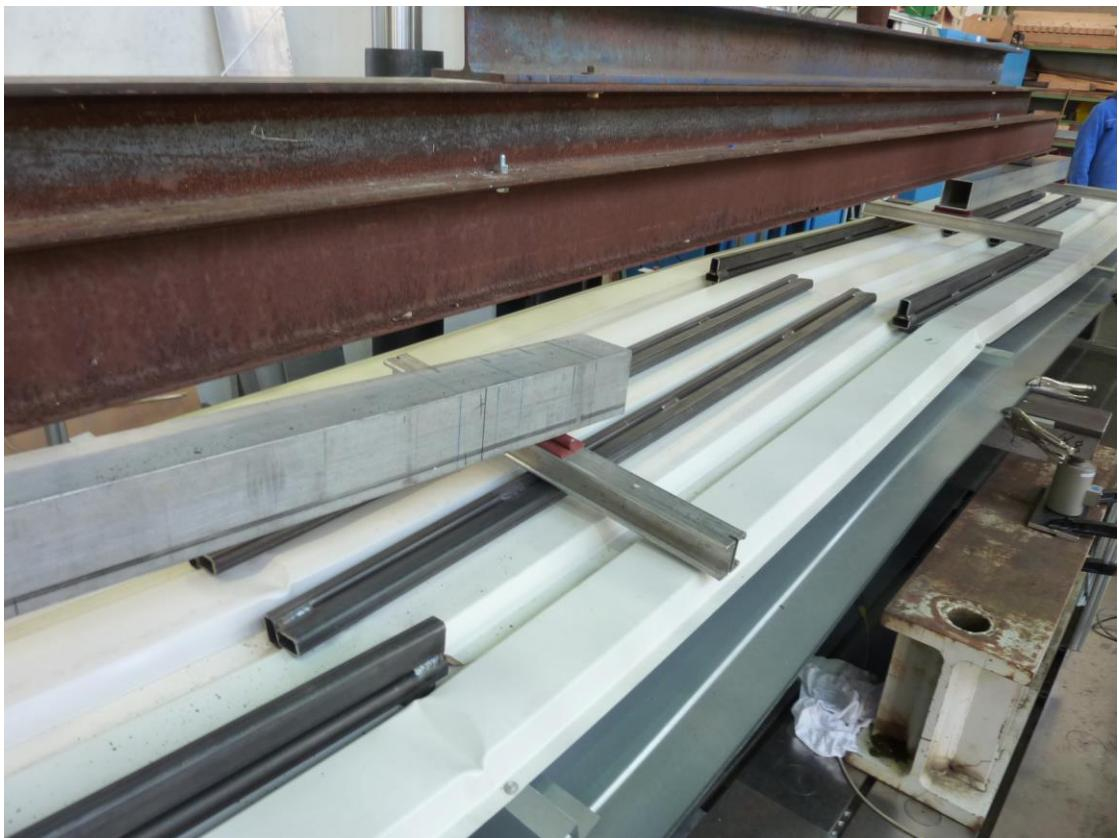
Figure D.8: Failure mode (buckling of the trapezoidal sheet in the middle of one span, Z-profile h = 50 mm)
