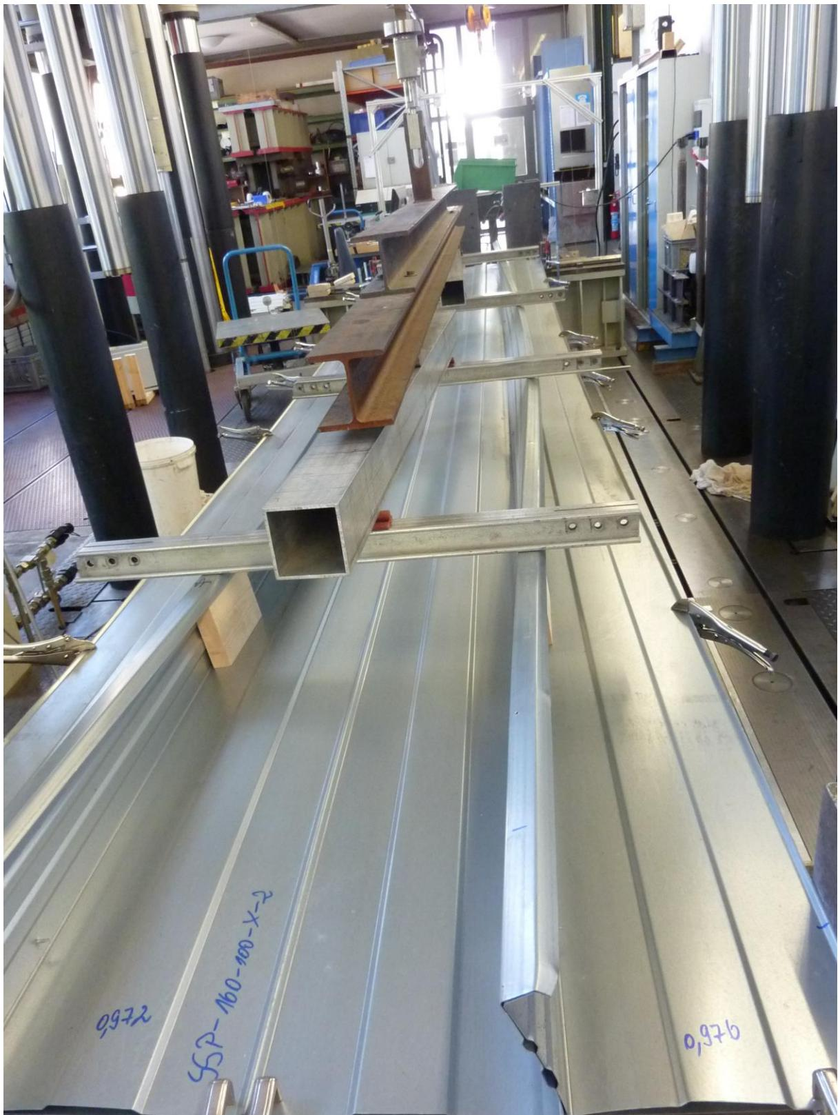
Figure B.10: Deformation of the upper flange and the web of the liner tray (liner tray without outer cladding, load distribution in the upper flange)
