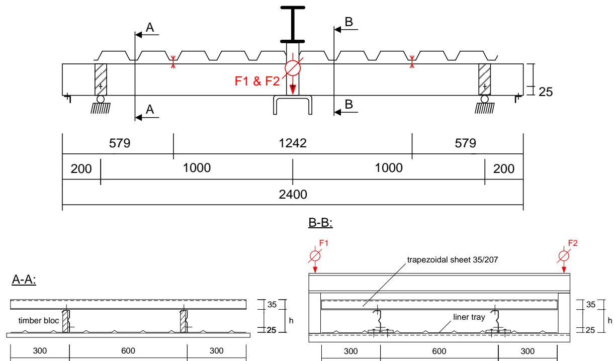
Figure C.2: Schematic test setup ( $s_1 = 1242$  mm)
