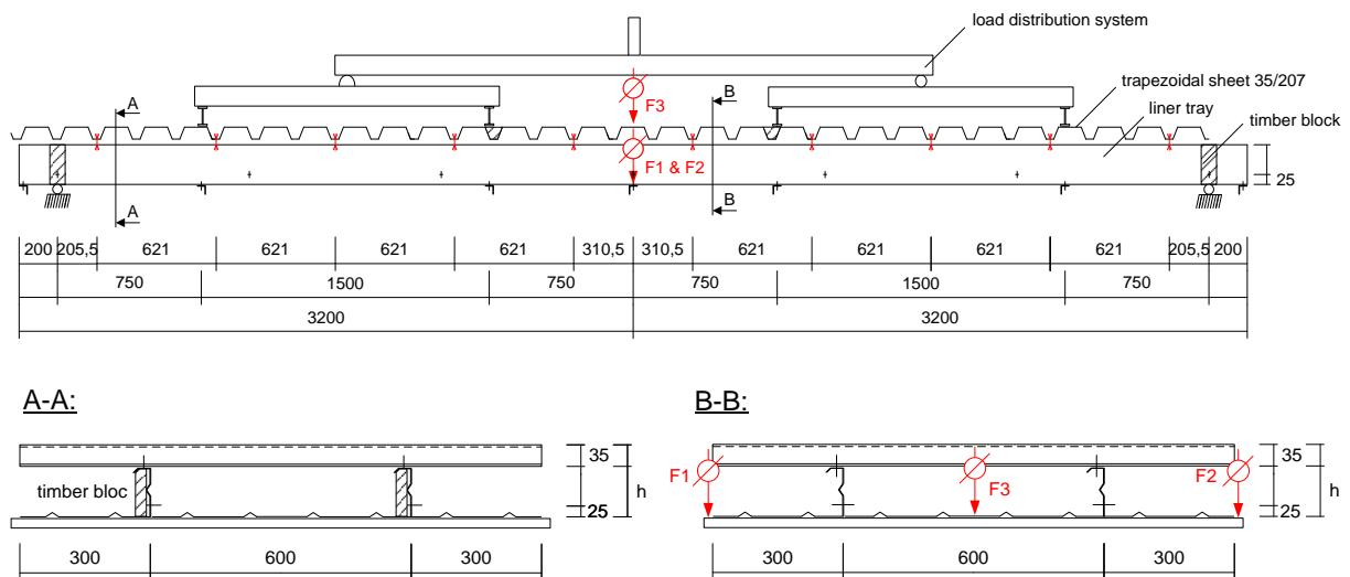
Figure B.1: Schematic test setup
