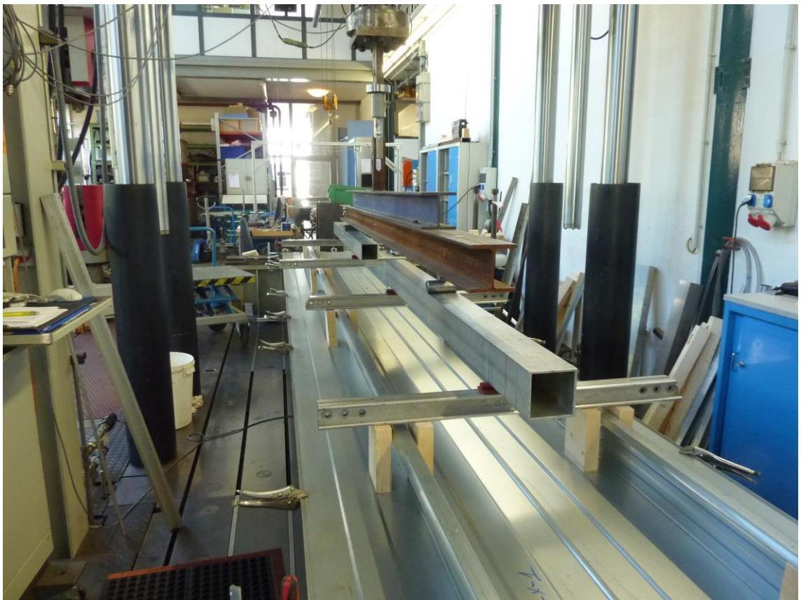
Figure B.7: Test setup (liner tray without outer cladding, load distribution in the lower flange)
