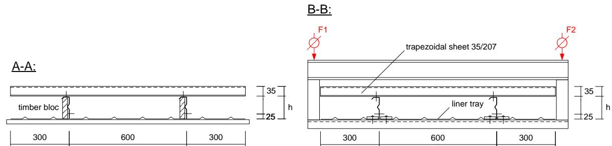
Figure C.1: Schematic test setup ( $s_1 = 621$  mm)
