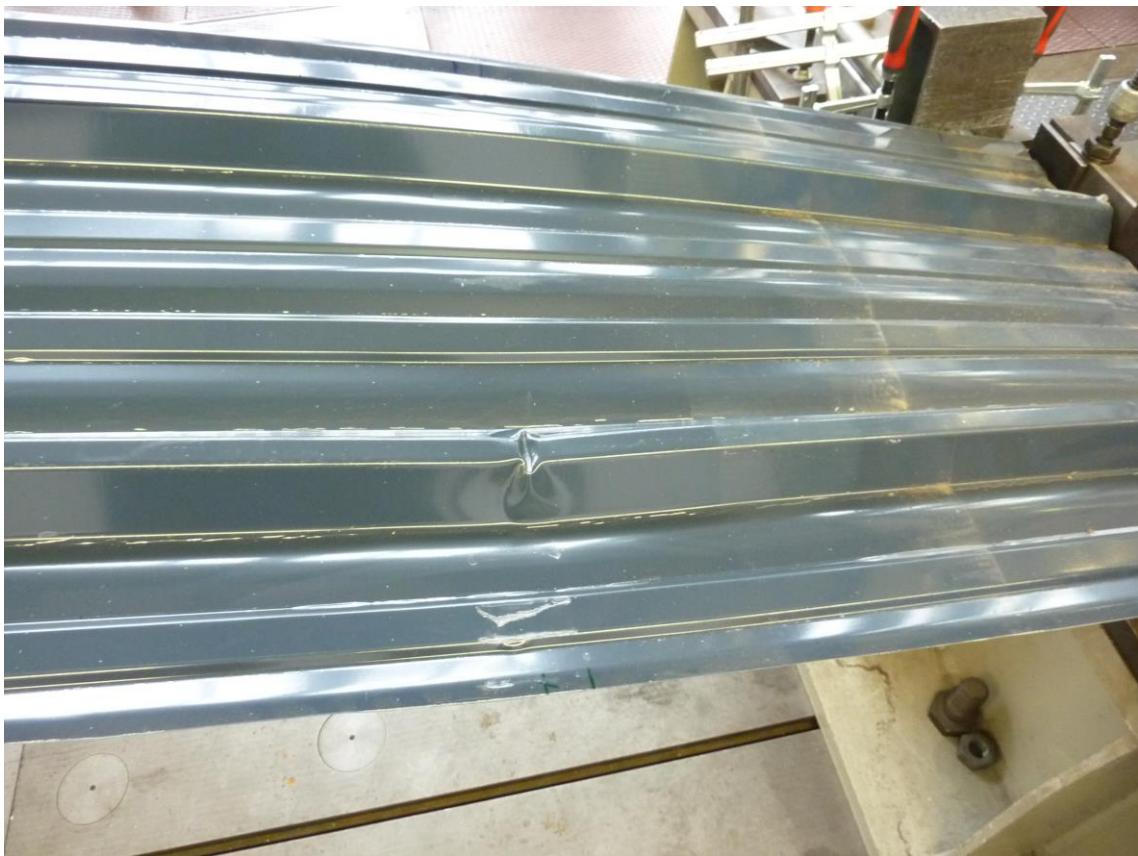
Figure C.7: Failure mode (local buckling) of SSP-H-576-063-1, detailed view
