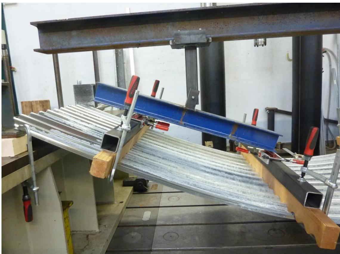
Figure B.8: Inclined position of load distribution beam of profile 18/76  $t_N = 1.00$  mm
