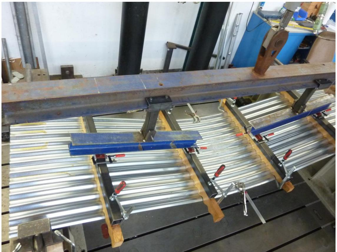
Figure B.9: Failure mode (plastic deformation) of profile 18/76  $t_N = 1.00$  mm with arch stitch  $h = 334$  mm
