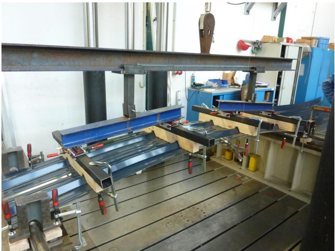
Figure B.5: Test setup for curved profiles, side view, exemplary for profile 39/333
