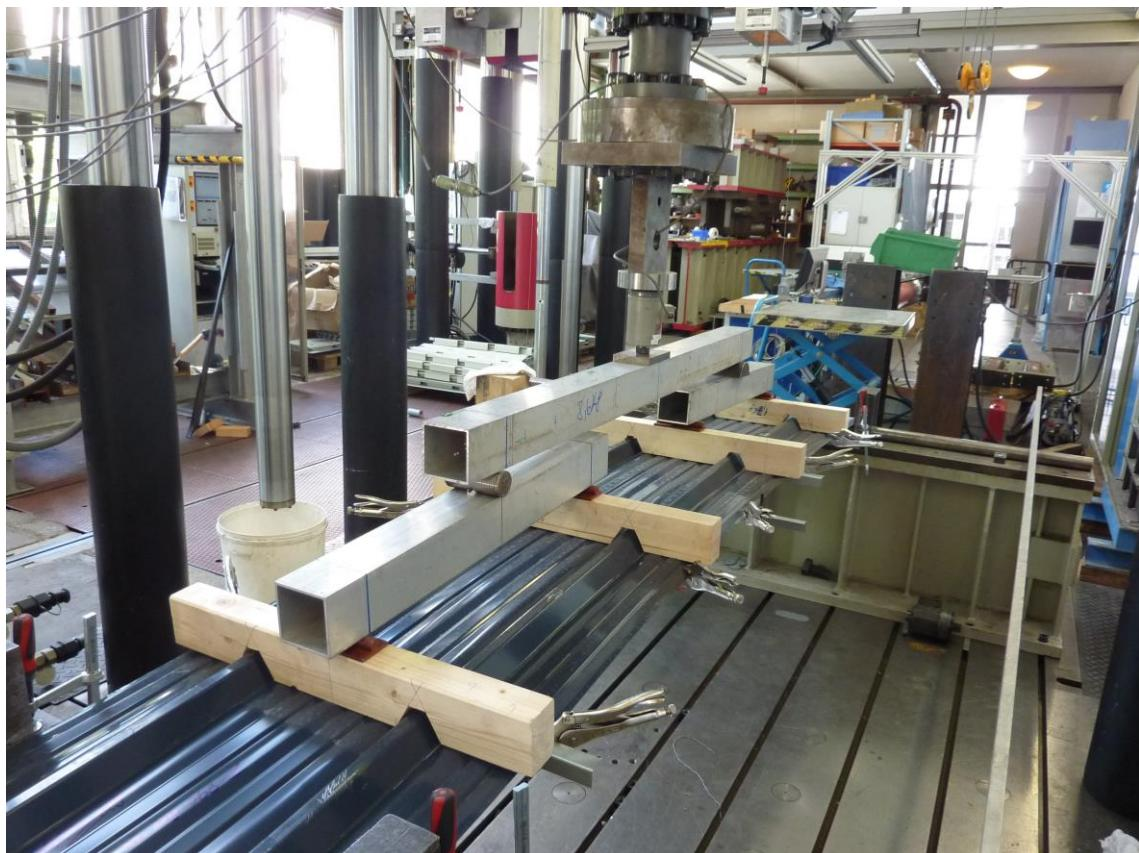
Figure B.2: Test setup for flat and profiles, side view, profile 39/333
