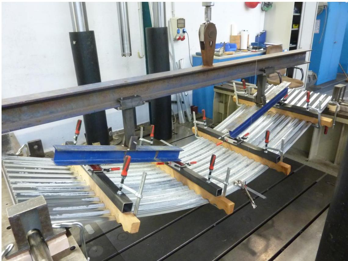
Figure B.7: Failure mode (plastic deformation) of profile 18/76  $t_N = 1.00$  mm
