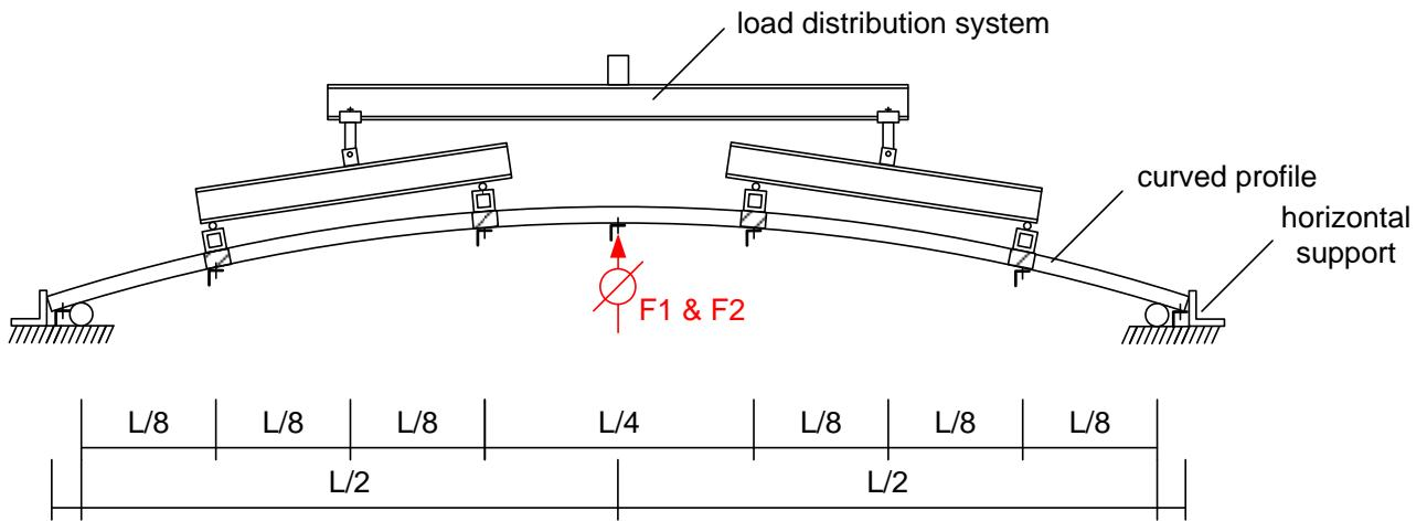
Figure C.1: Schematic test setup
