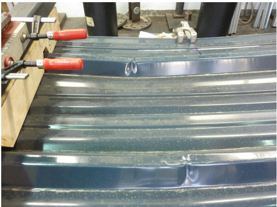
Figure B.11: Failure mode (local buckling of the upper flange), detailed view
