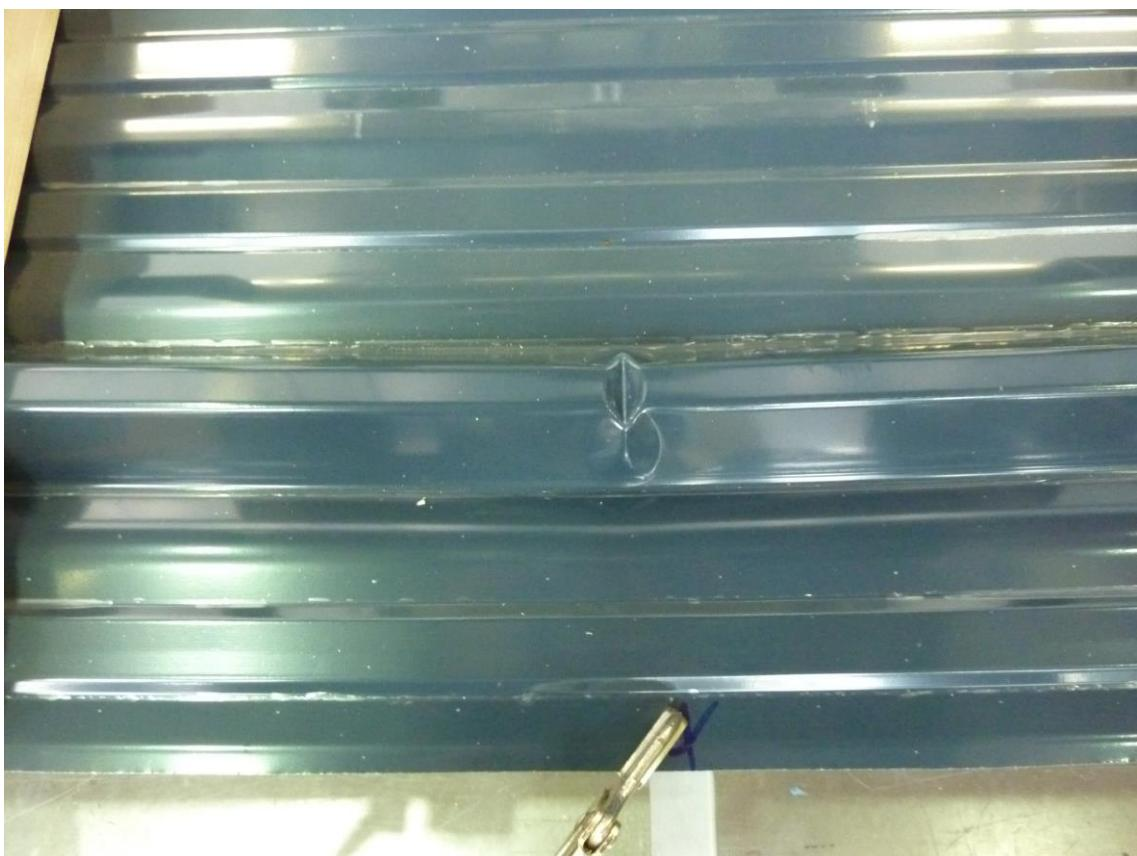
Figure B.10: Failure mode (local buckling of the upper flange) of profile 39/333
