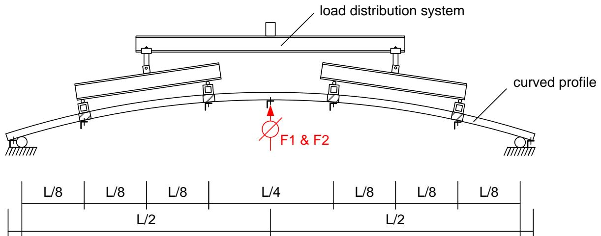
Figure B.1: Schematic test setup
