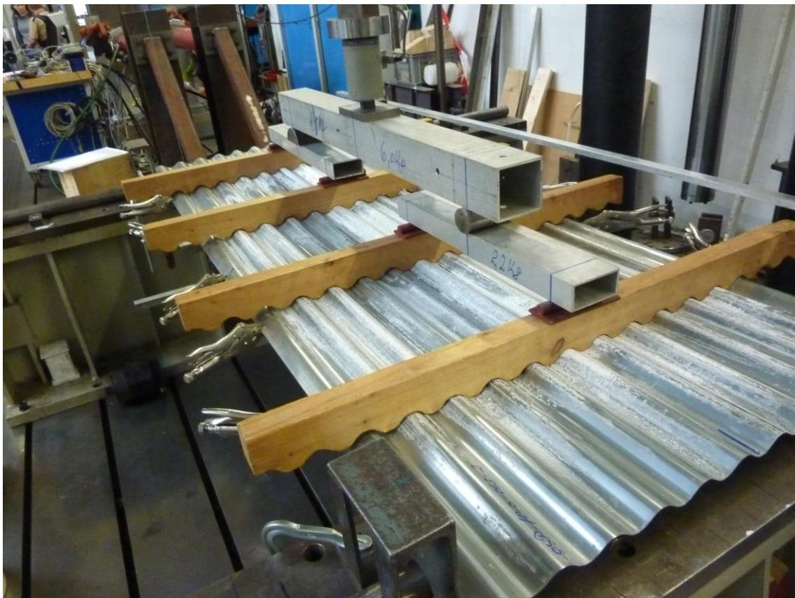
Figure B.3: Test setup for flat profiles, side view, profile 18/76
