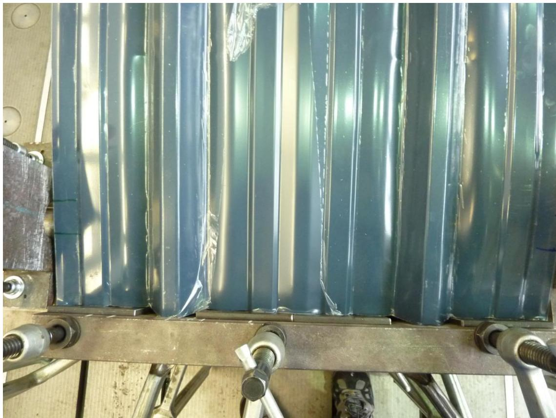
Figure C.3: Plastic deformation at the support
