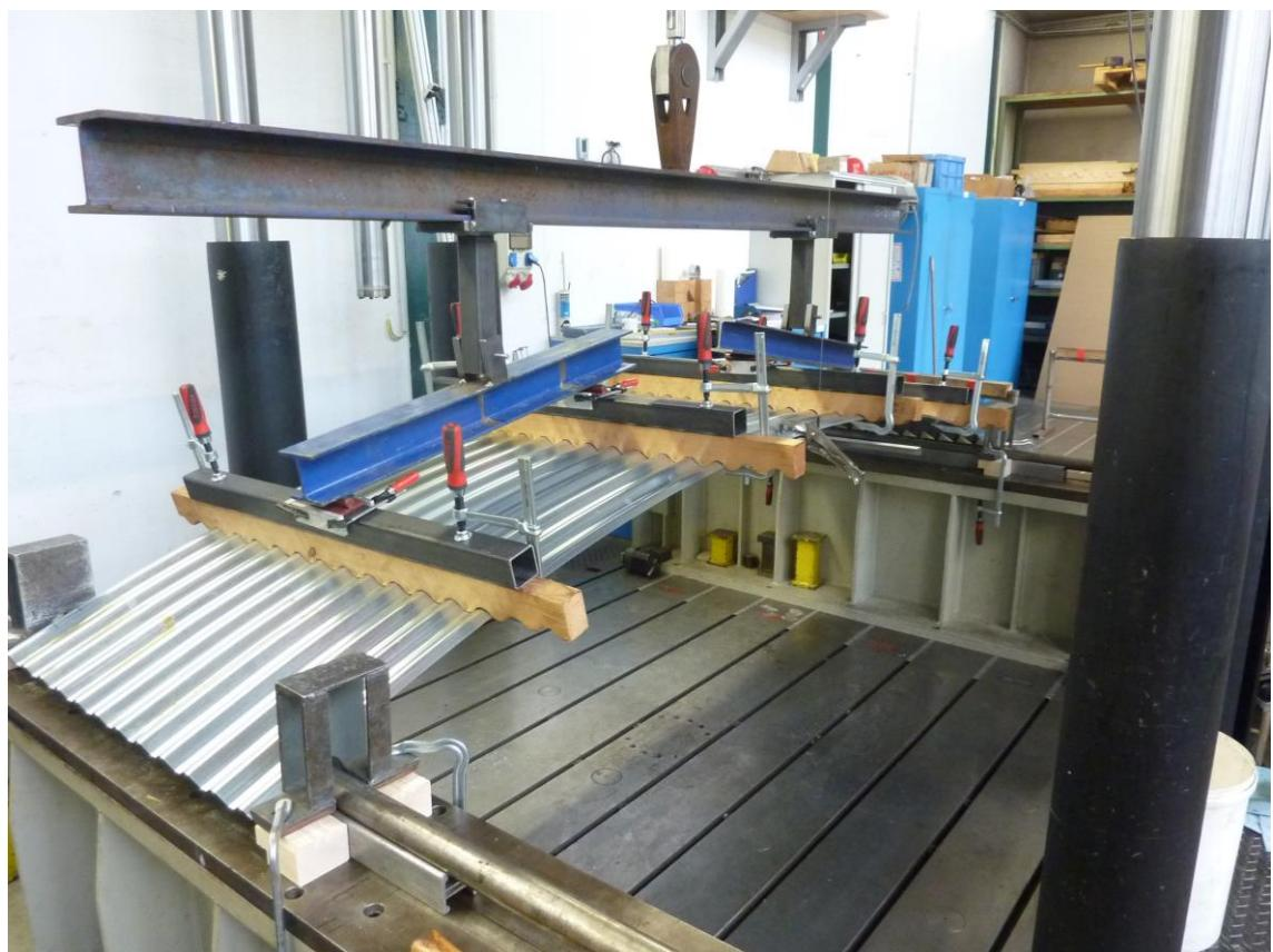
Figure B.4: Test setup for curved profiles, side view, exemplary for profile 18/76
