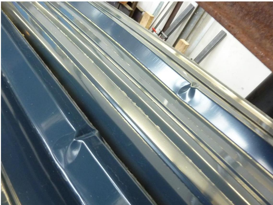
Figure C.8: Failure mode (local buckling) of SSP-H-576-063-2 and SSP-H-576-063-3
