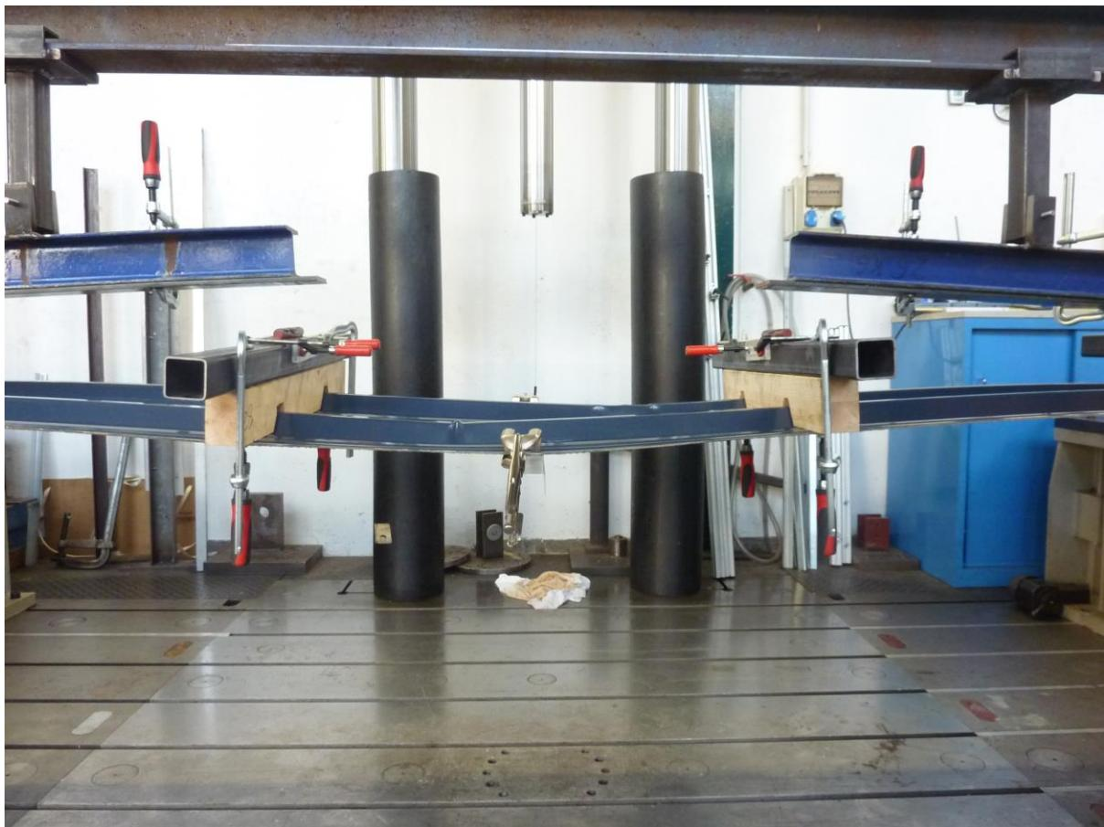
Figure B.12: Failure mode (local buckling of the upper flange) of profile 39/333 with arch stitch  $h = 380$  mm
