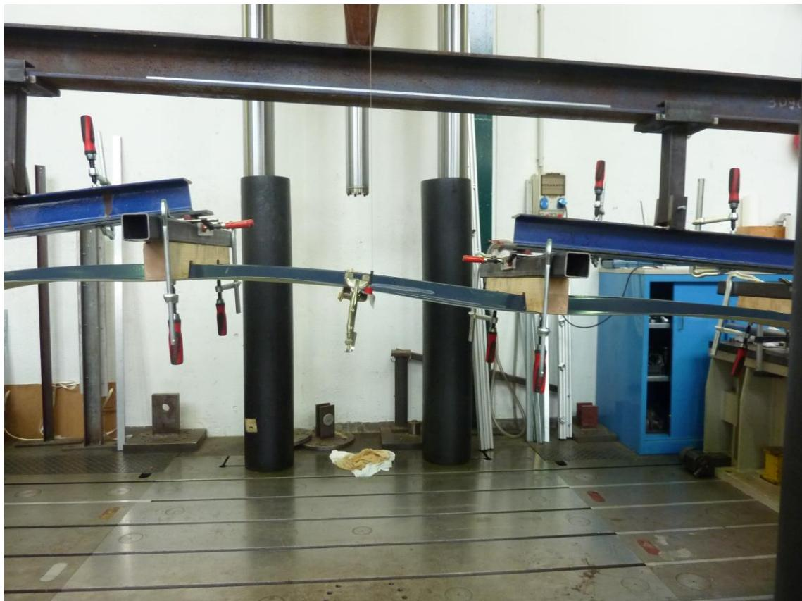
Figure C.4: Failure mode (buckling of the arch) for arch stitich  $h = 217$  mm and  $h = 380$  mm
