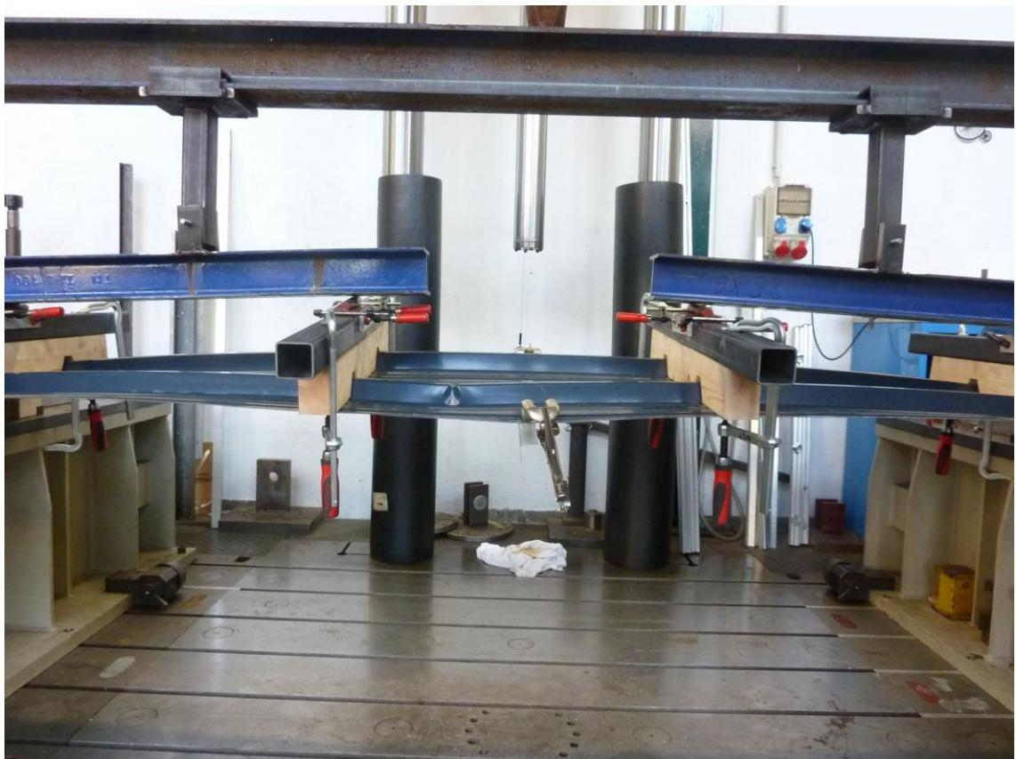
Figure B.10: Failure mode (local buckling of the upper flange) of profile 39/333 with arch stitch  $h = 217$  mm
