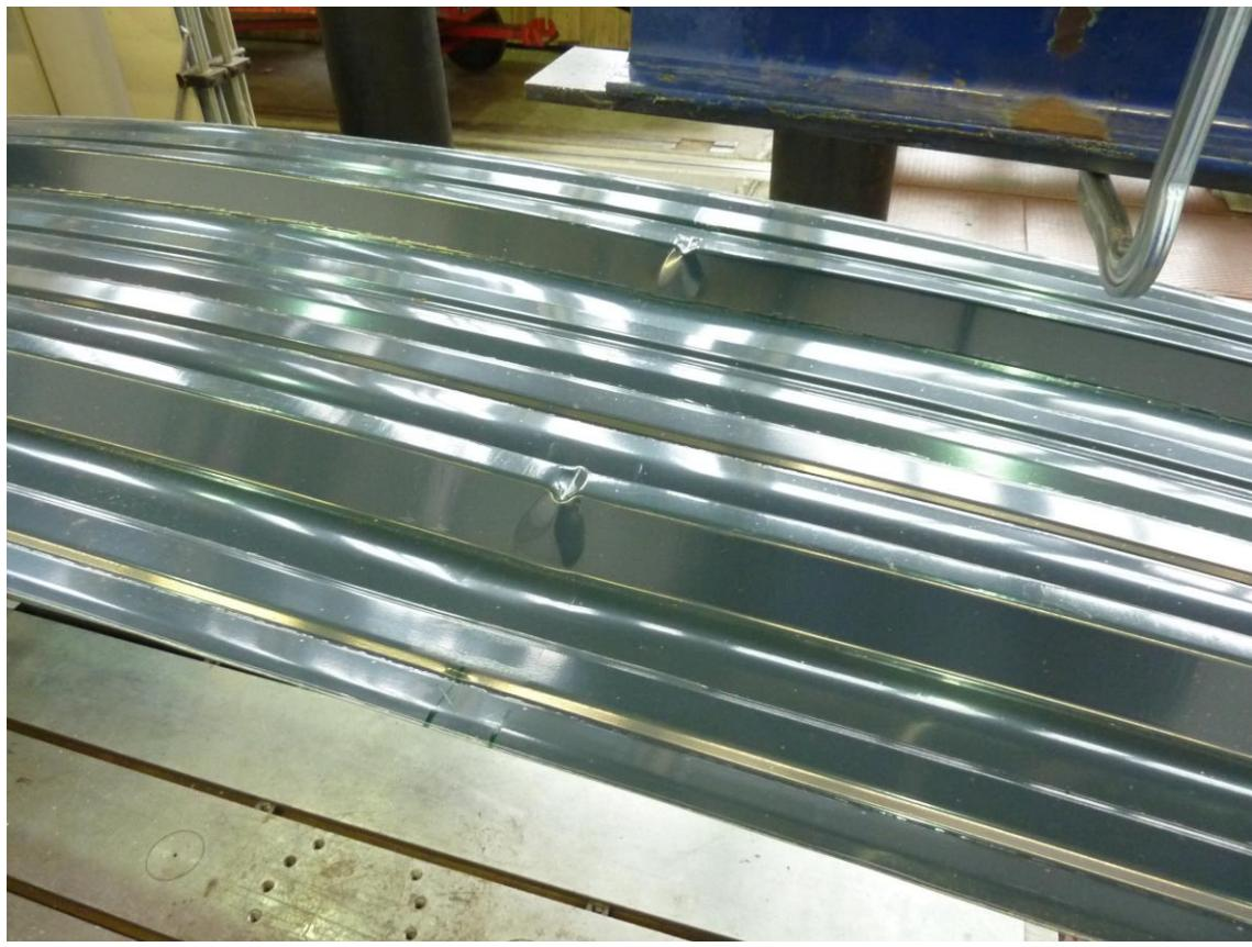
Figure C.5: Failure mode (local buckling) for arch stitch  $h = 217$  mm and  $h = 380$  mm
