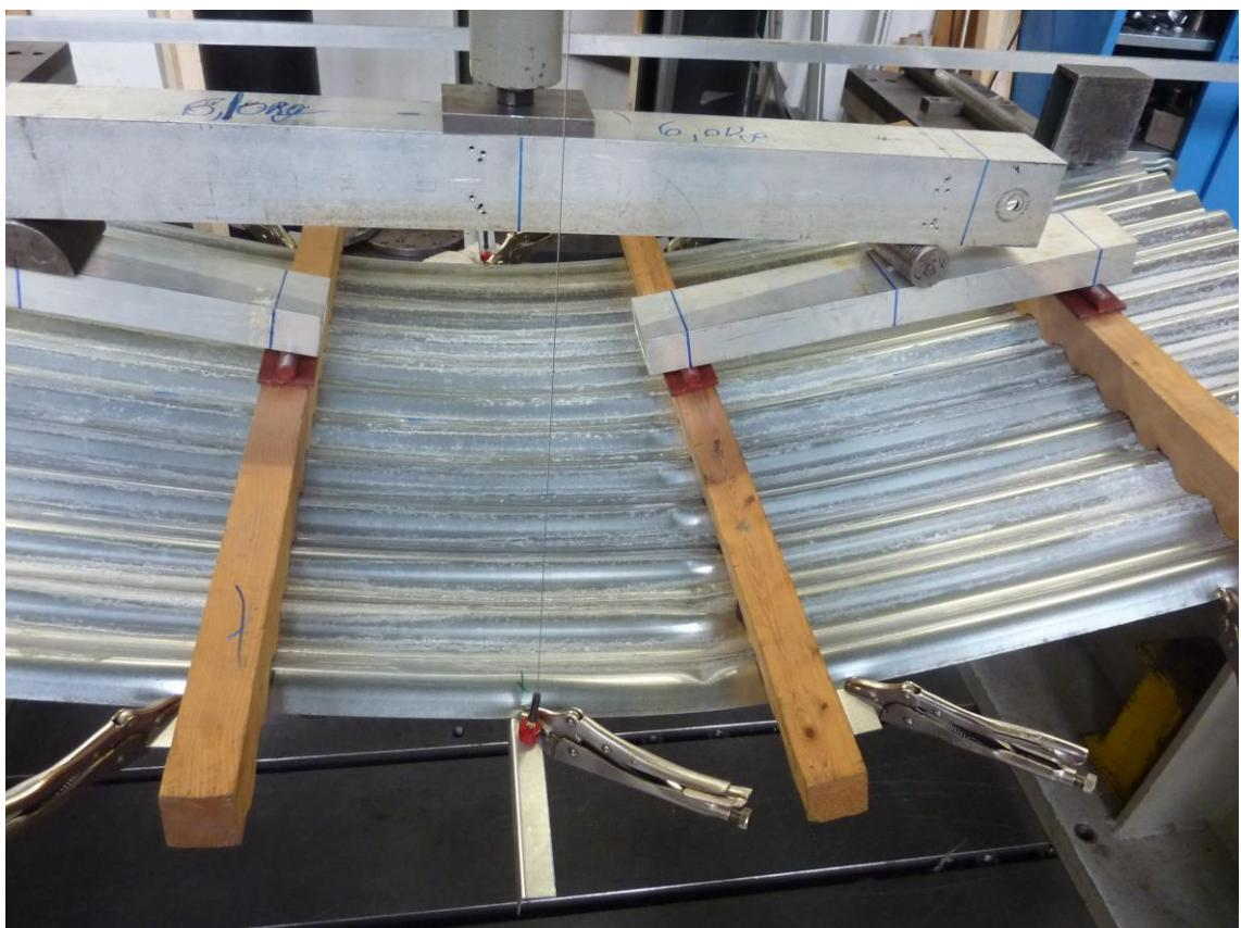
Figure B.6: Failure mode (local buckling) of profile 18/76  $t_N = 0.63 \text{ mm}$
