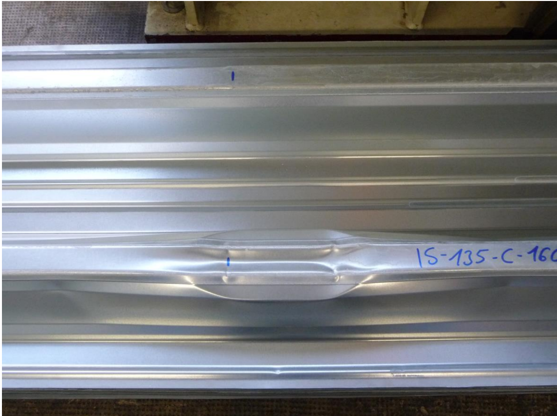
Figure B.6: Failure mode (exemplary IS-135-C-160-75-80-1)
