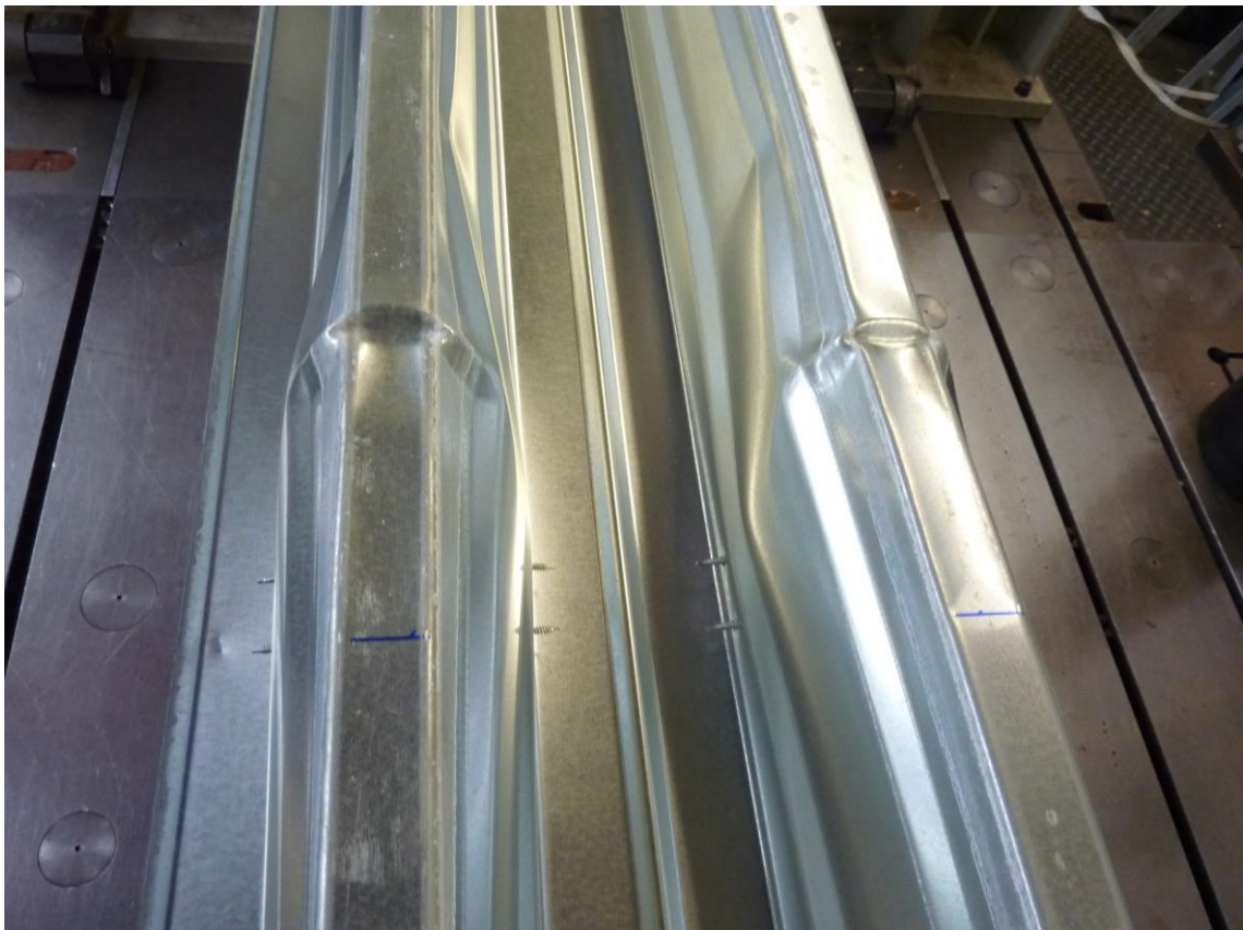
Figure B.37: Failure mode (exemplary IS-158-CR-160-100-320-2)
