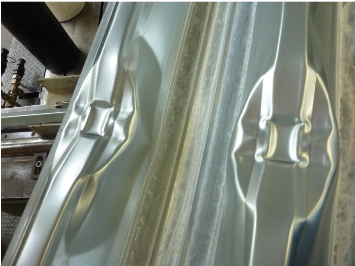
Figure B.5: Failure mode (exemplary IS-135-C-60-75-280-2)
