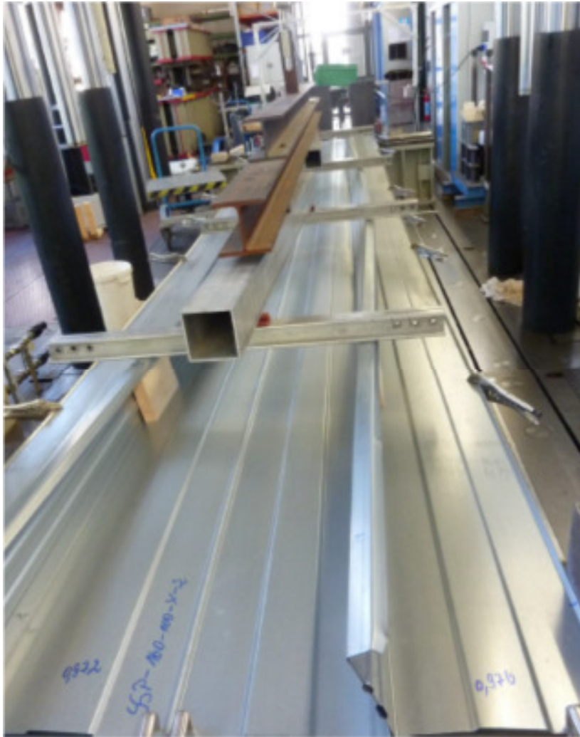
Fig. 8: Single span test without outer cladding
