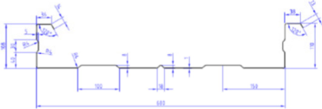
Fig. 2: Cross section of the liner tray JID 110/600
