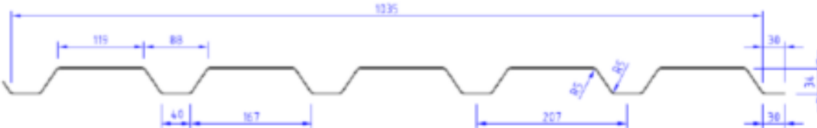
Fig. 4: Cross section of the trapezoidal sheeting JID 35/207
