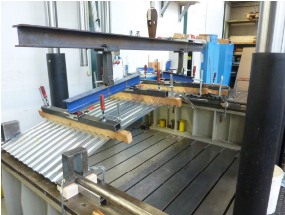
Fig. 6: Real setup of the single span tests without horizontal support
