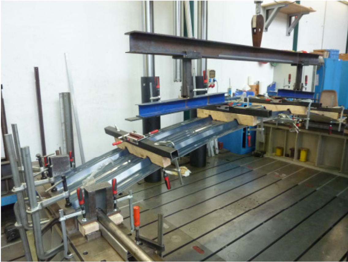
Fig. 9: Real setup of the arch tests
