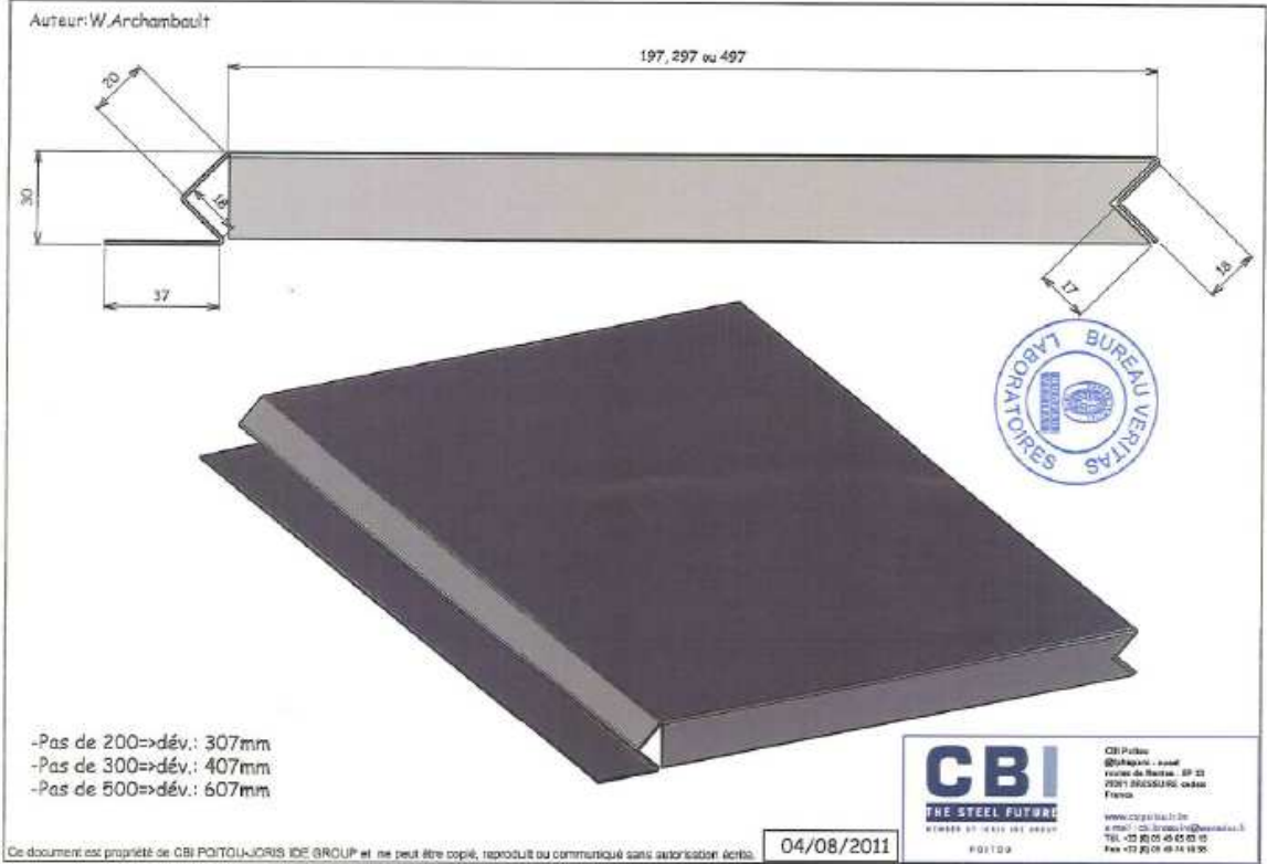
Figure 7: Geometry of ZEPHIR 300
