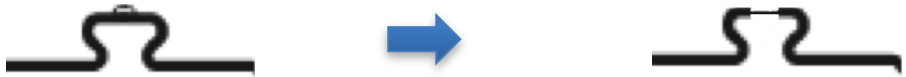
Fig. 3.3.1 – Upper part of the outwards stiffener with a reduced thickness replacing the embossment
