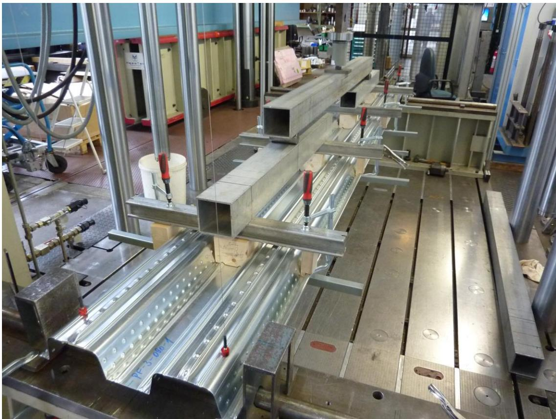
Figure B.4: Test setup (exemplary for ComFlor80,  $t_N = 0.90$  with outward stiffeners)
