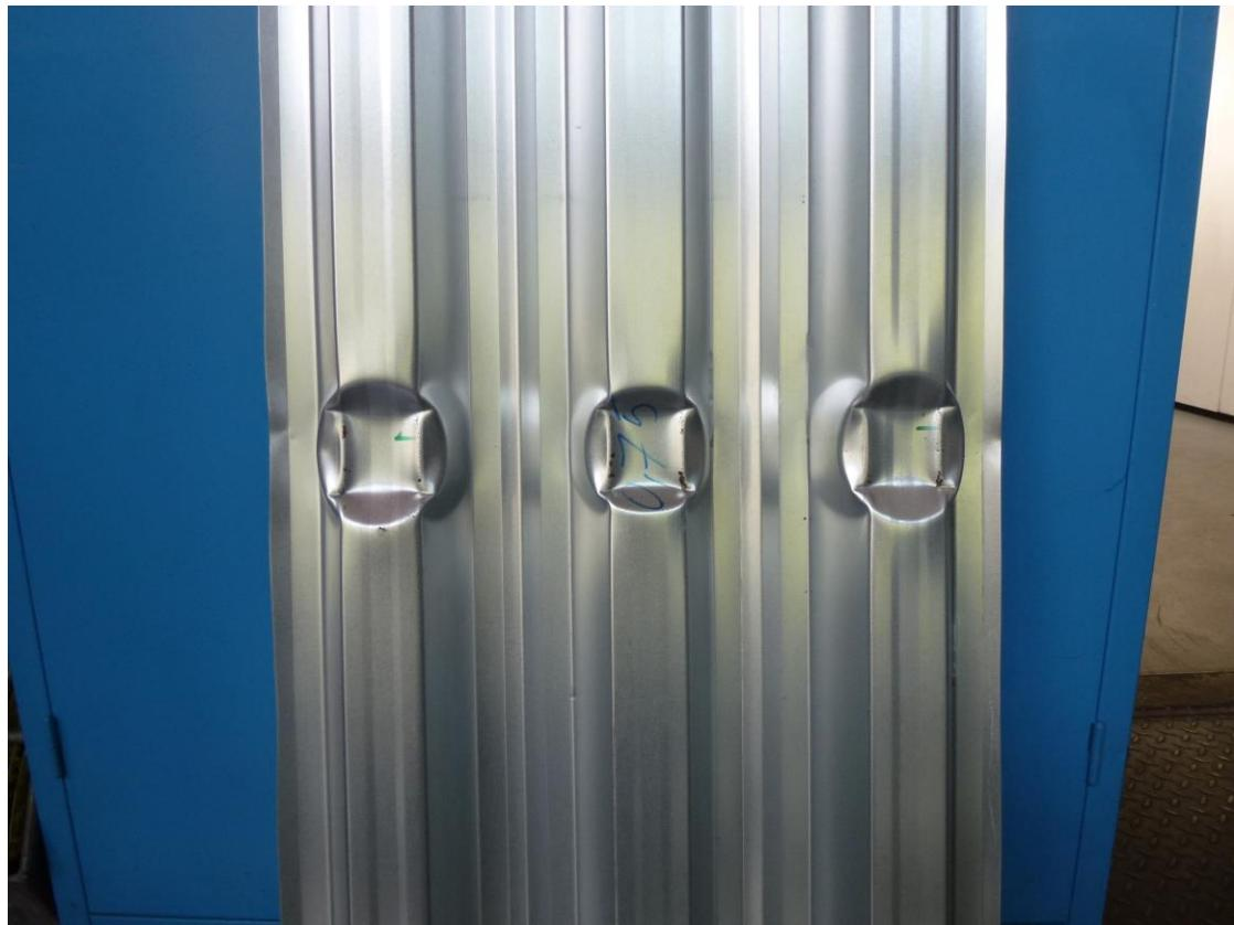
Figure C.4: Failure mode (exemplary for PCB 80,  $b_u = 60$  mm,  $t_N = 0.75$  without embossments)
