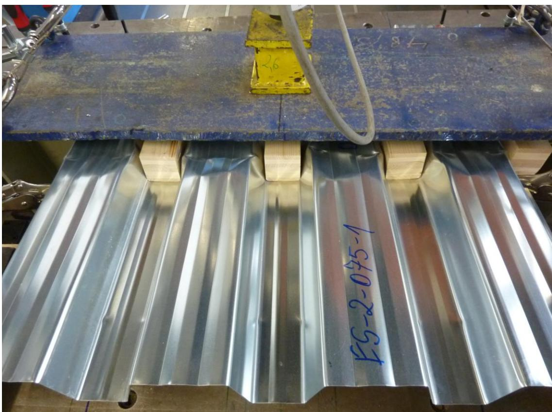
Figure D.12: Buckling of the upper flanges (PCB 60,  $t_N = 0.75$  mm without embossments)
