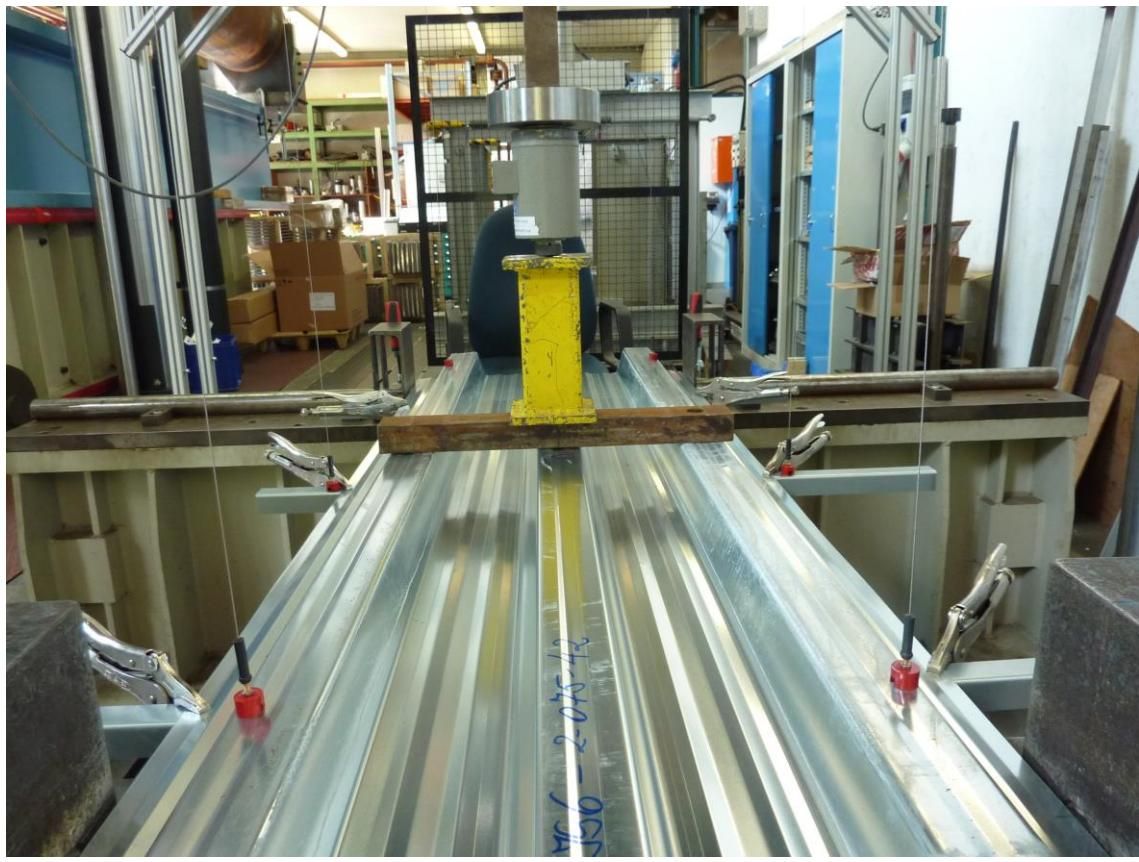
Figure C.3: Test setup (exemplary for PCB 60,  $b_u = 60$  mm,  $t_N = 0.75$  mm without embossments)
