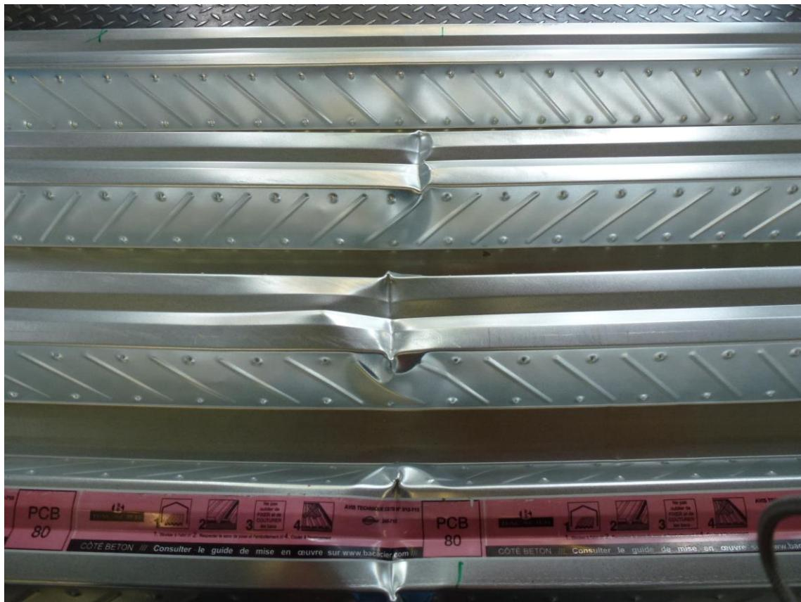
Figure B.6: Failure mode (PCB 80,  $t_N = 0.75$  mm with embossments)
