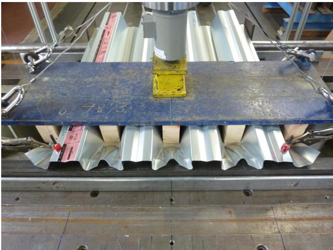
Figure D.4: Web-crippling (PCB 80  $t_N = 0.75$  mm without embossments)
