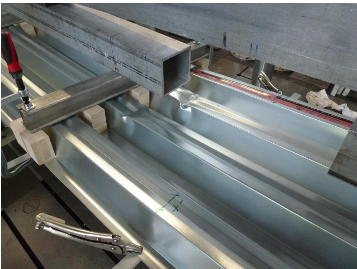
Figure B.5: Failure mode (PCB 80  $t_N = 0.75$  mm without embossments)
