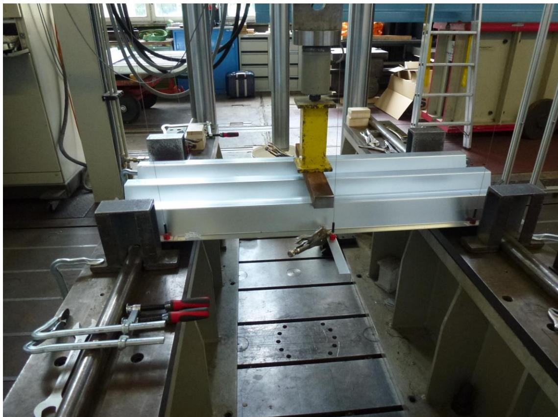
Figure C.2: Test setup (exemplary for PCB 80,  $b_u = 60$  mm,  $t_N = 0.75$  mm without embossments)
