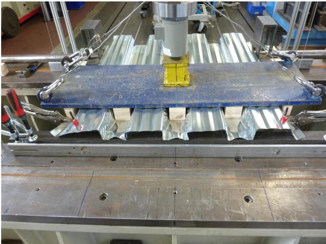
Figure D.16: Web-crippling (PCB 60  $t_N = 0.75$  mm with embossments)
