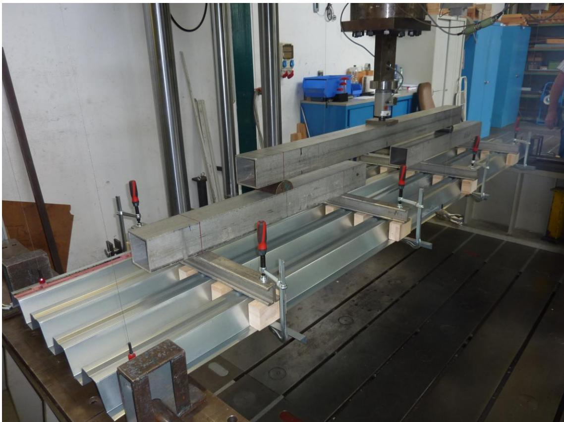
Figure B.2: Test setup (exemplary for PCB 80,  $t_N = 1.00$  mm without embossments)
