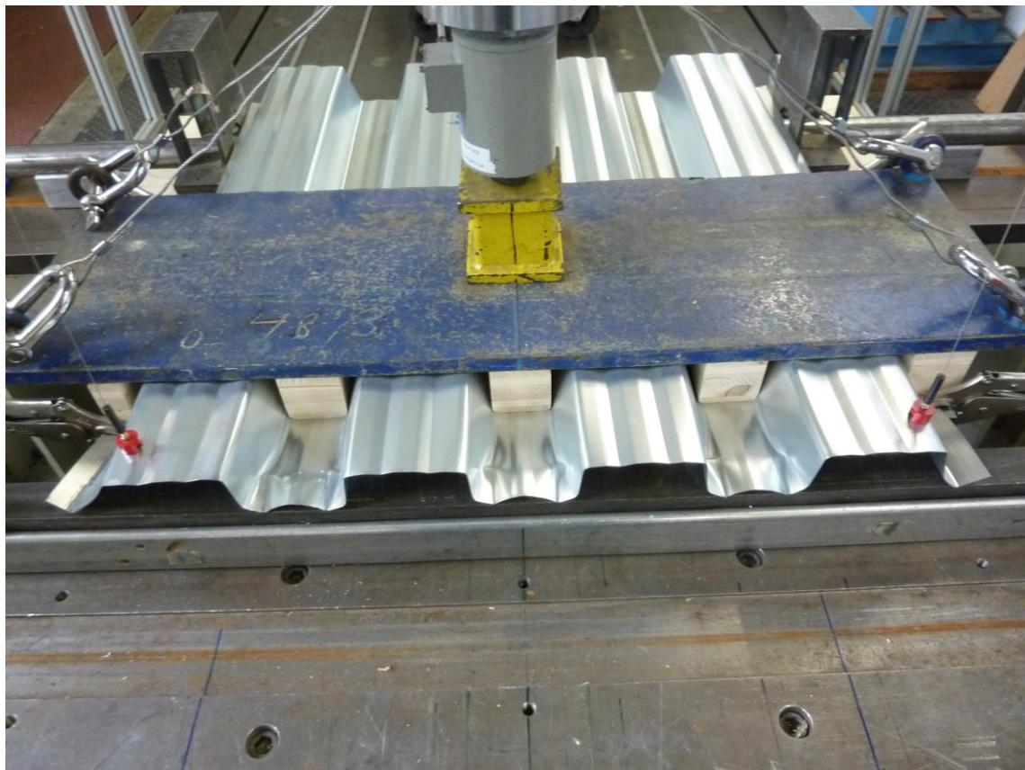
Figure D.13: Web-crippling (PCB 60  $t_N = 1.00$  mm without embossments)
