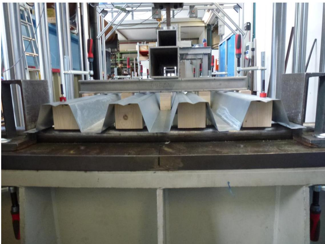
Figure B.3: Test setup (exemplary for PCB 80,  $t_N = 1.00$  mm without embossments)
