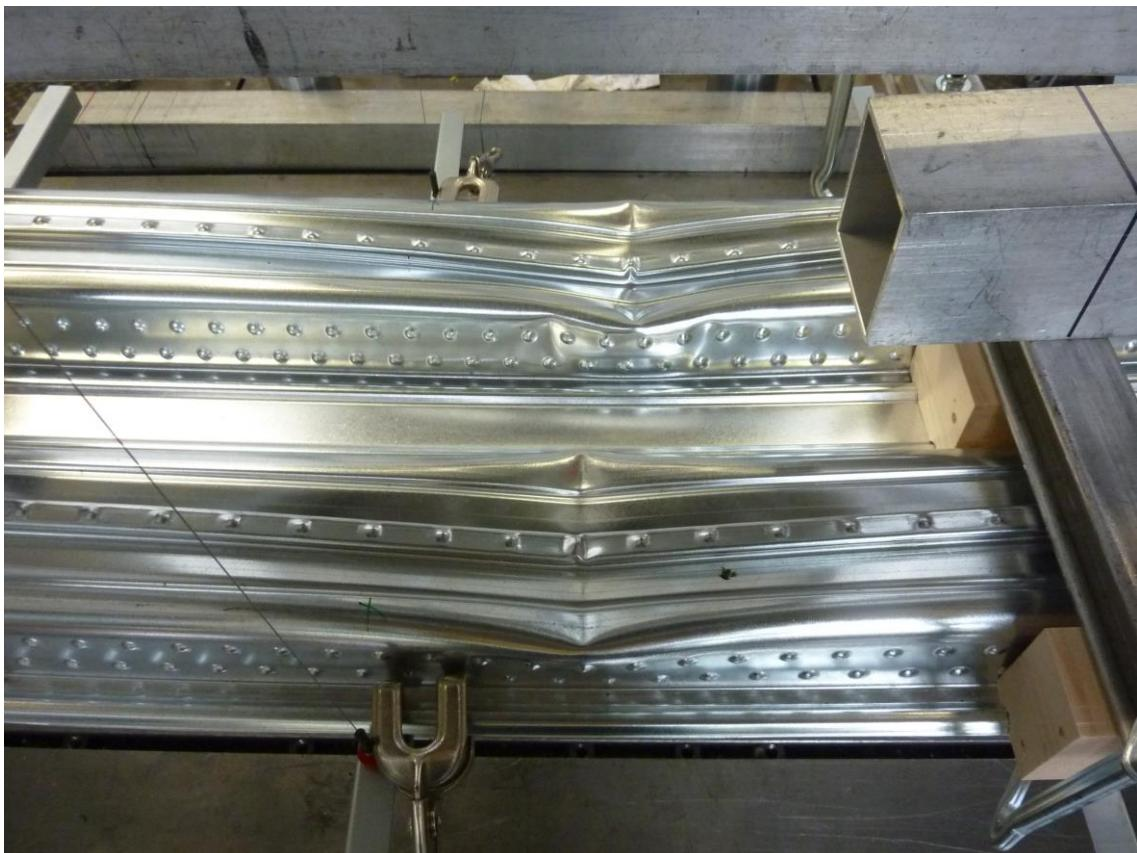
Figure B.9: Failure mode (ComFlor 80,  $t_N = 0.90$  mm with outward stiffeners)
