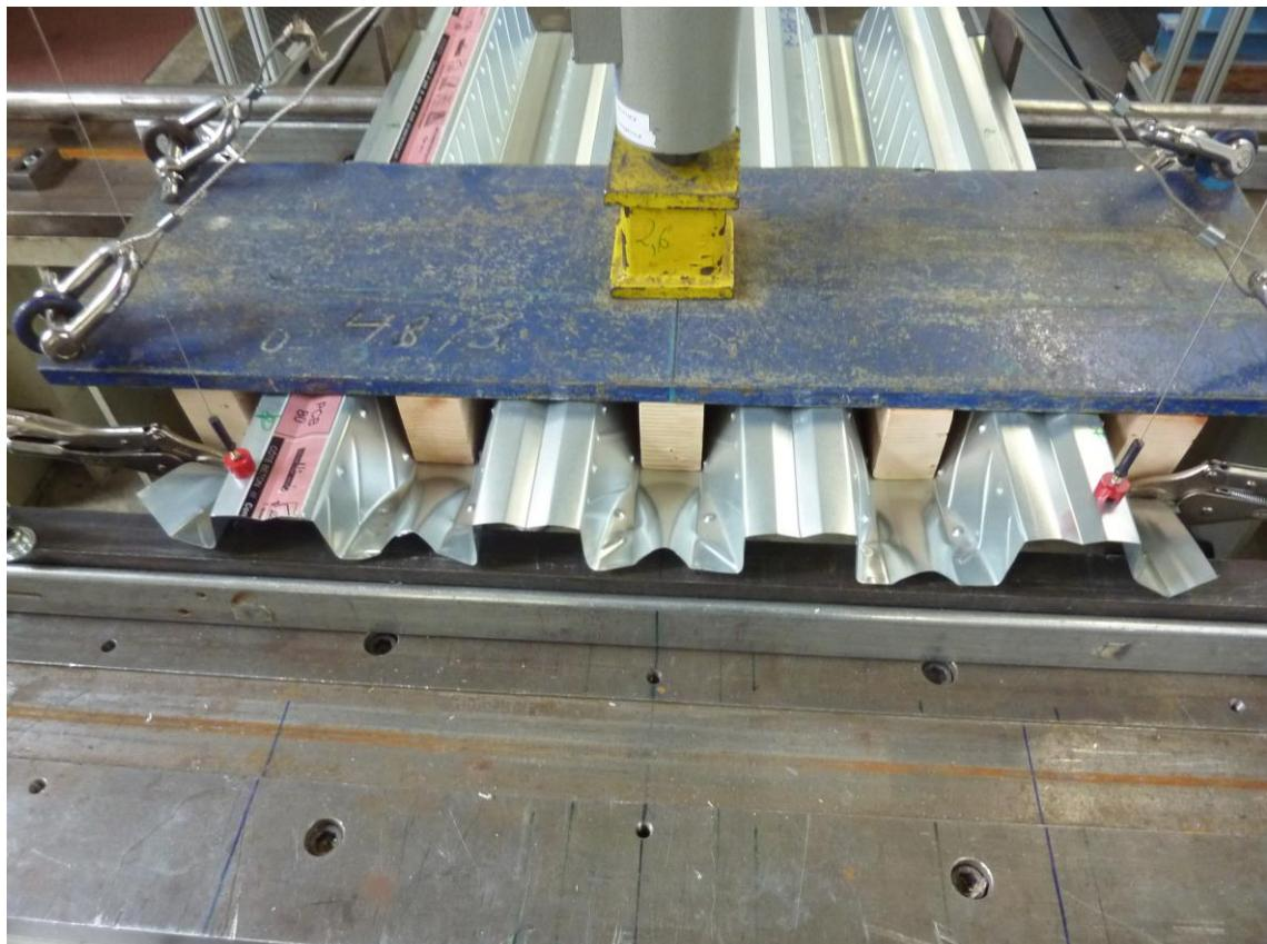
Figure D.6: Web-crippling (PCB 80  $t_N = 0.75$  mm with embossments)
