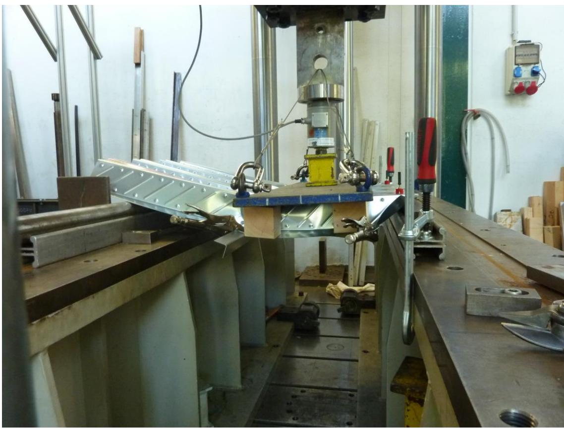
Figure D.9: Deformation at the end of the test (PCB 80,  $t_N = 0.75$  mm with embossments)
