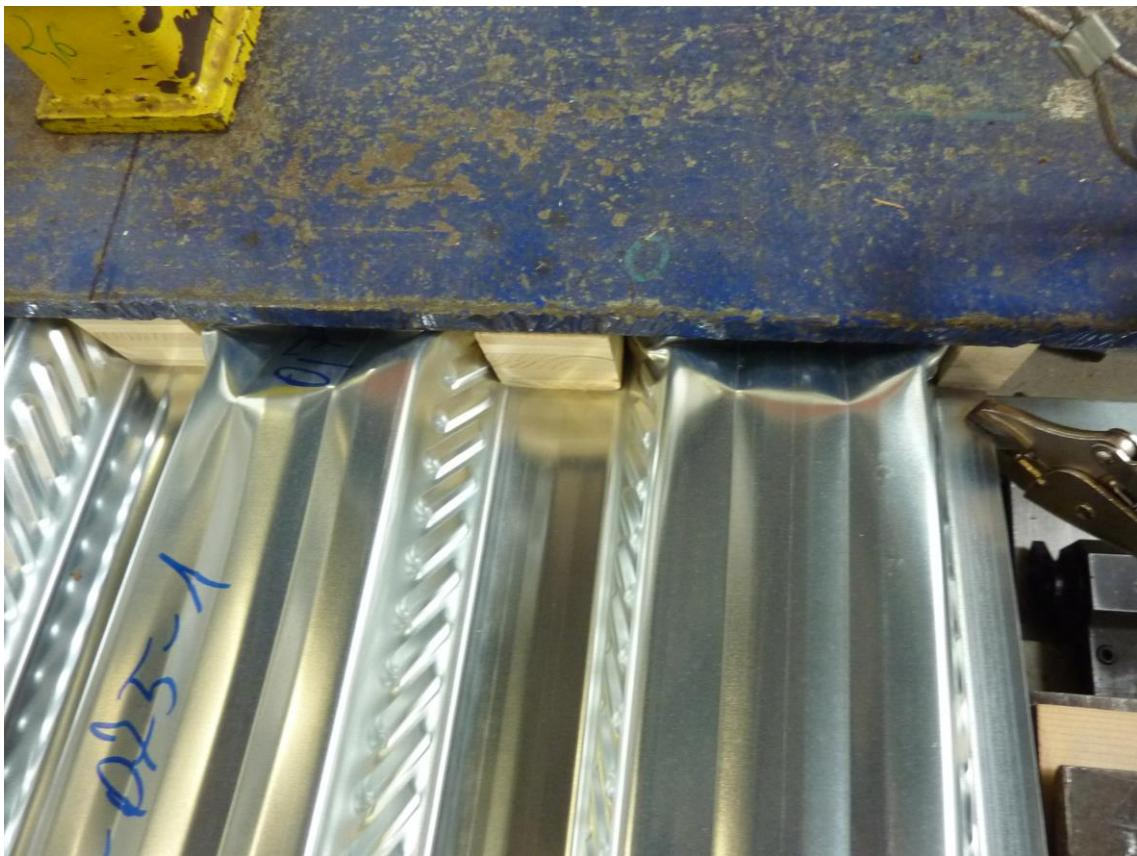
Figure D.17: Buckling of the upper flanges (PCB 60,  $t_N = 0.75$  mm with embossments)
