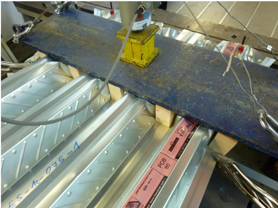
Figure D.8: Buckling of the upper flanges (PCB 80,  $t_N = 0.75$  mm with embossments)
