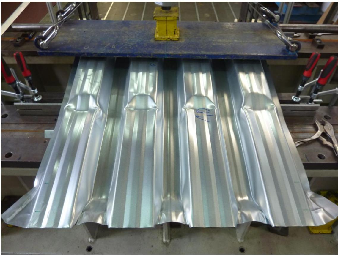
Figure D.15: Buckling of the upper flanges (PCB 60,  $t_N = 1.00$  mm without embossments, test 3)
