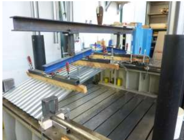
Figure 1-9: Picture of the test setup single span tests.
