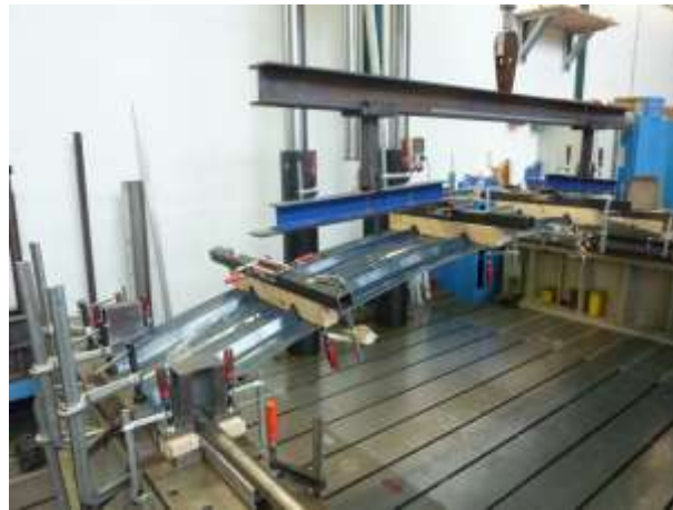
Figure 1-11: Picture of the test setup single span test with horizontal support (profile 39/333).
