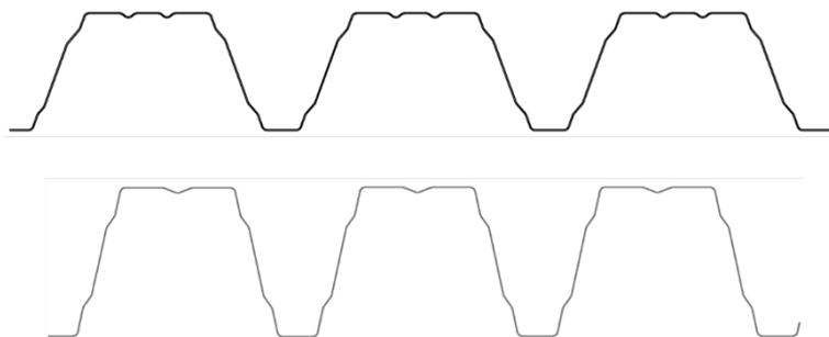
Figure 10 - Typical geometries of profiled steel sheets
