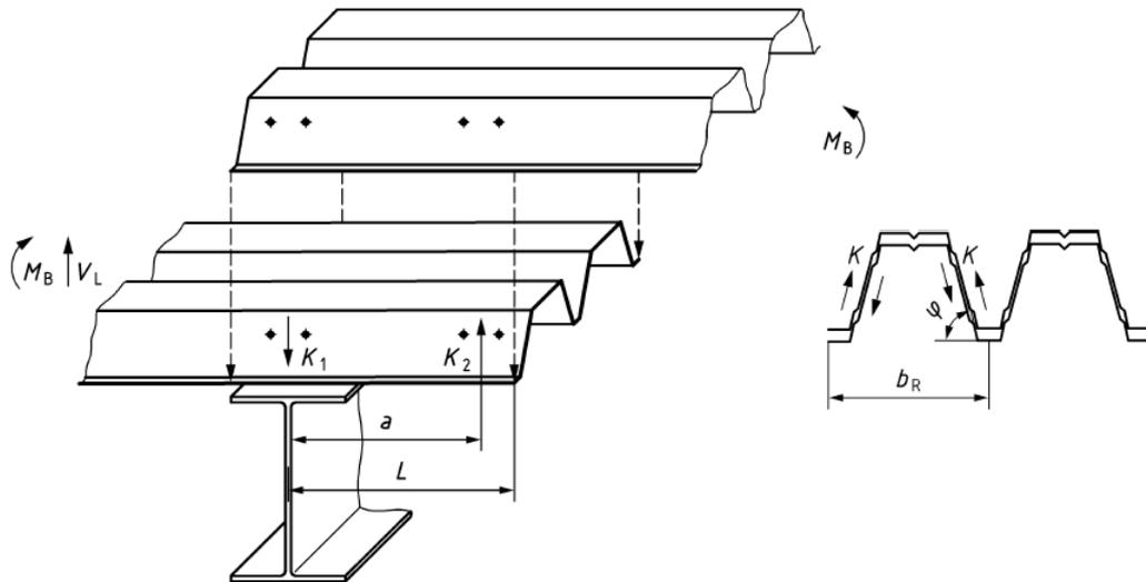
Figure 2 – Overlapped profiles in accordance with standard [4] and with the end of the profile cantilevered below
