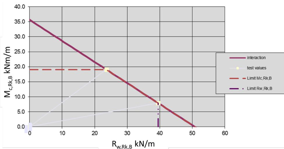
Figure 8 - Example of an interaction diagram obtained from 2 intermediate support tests.
