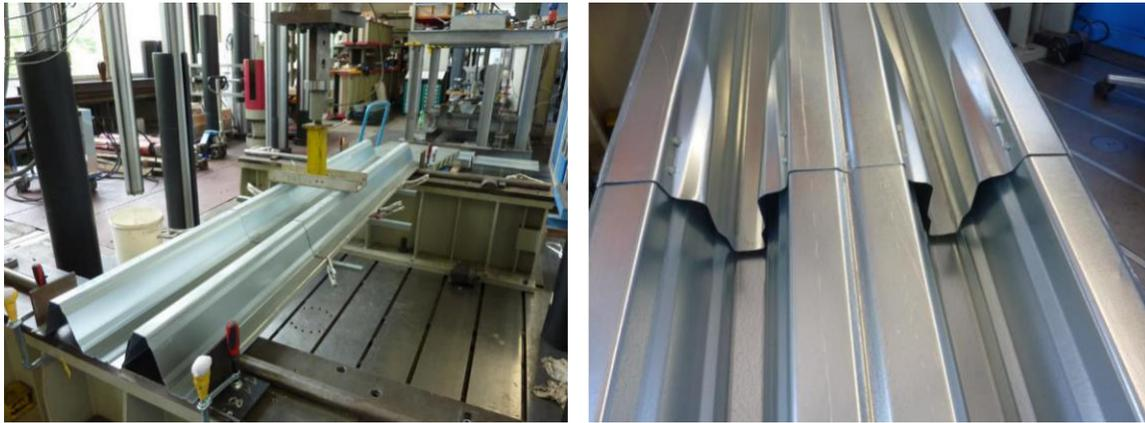
Figure 7 - Example of connection failure in an intermediate bearing test
