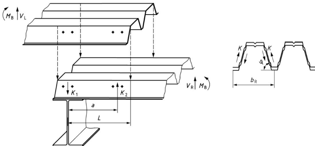
Figure 3 - Overlapped profiles in accordance with standard [4] with the end of the profile cantilevered above.
