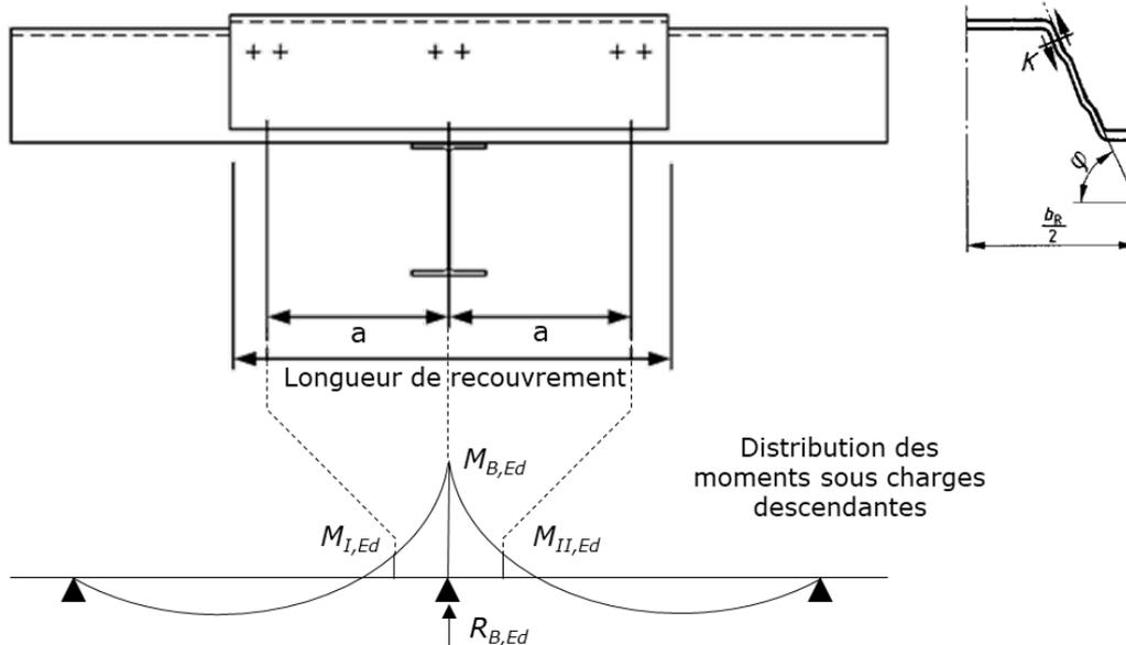
Figure 12 - Continuous profile with local reinforcement
