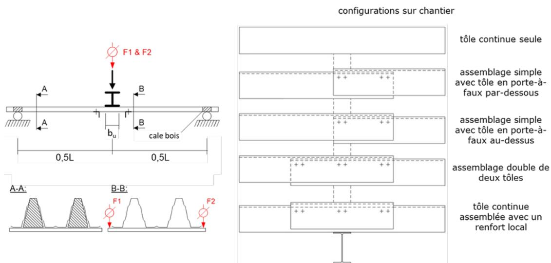
Figure 6 - Schematic principle of the intermediate support test
