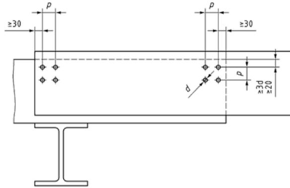
Figure 4 - Fastener layout according to standard [4] for efficient assembly.
