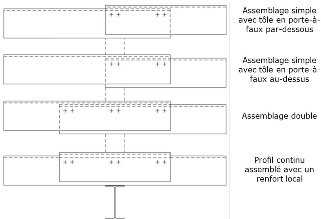
Figure 1 – Assemblies of profiled steel sheets on intermediate support
