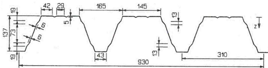
Figure 13 - profile 137-310-930 in positive position (normal position).
